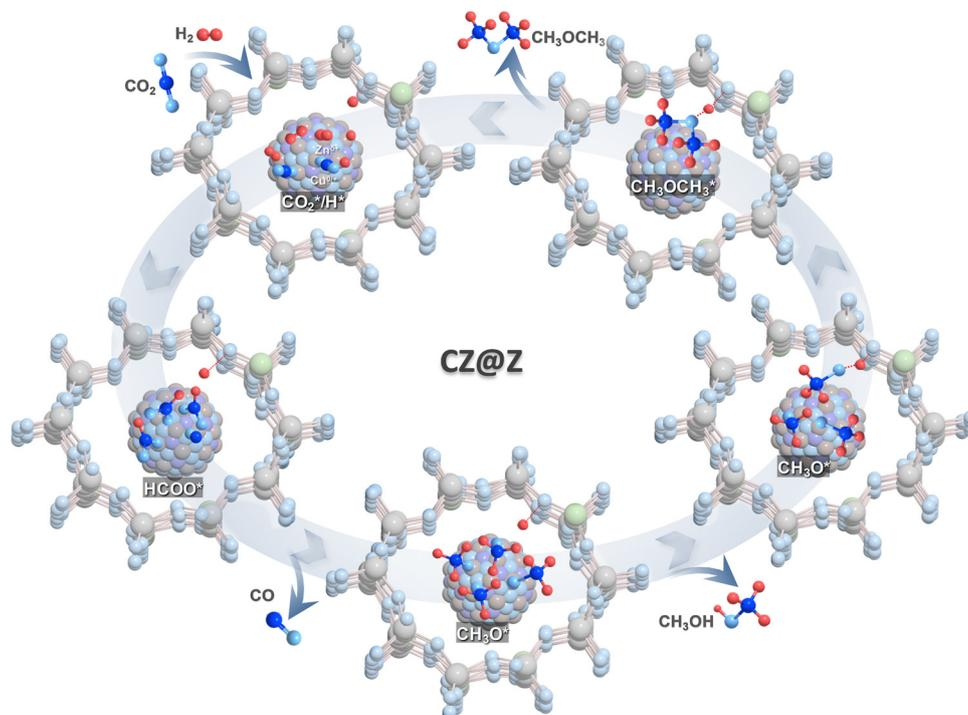
Fig. 9 Proposed reaction mechanisms for direct CO<sub>2</sub> hydrogenation to DME and methanol over ZSM-5-encapsulated Cu–ZnO nanoparticles.
