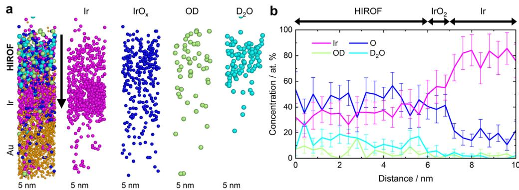
Fig. 5 Atomic interface analysis post-HIROF formation on 2 nm thick film. (a) 2D interface analysis. (b) 1D concentration profiles (OD, D<sub>2</sub>O, Au, and Ir) after 500 cycles.
