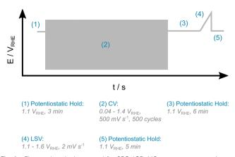
$\label{eq:Fig.1} \textbf{Fig. 1} \quad \textbf{Electrochemical protocol for SFC-ICP-MS measurements to investigate HIROF growth.}$
