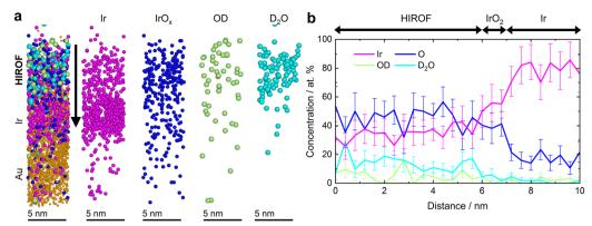
Fig. 5 Atomic interface analysis post-HIROF formation on 2 nm thick film. (a) 2D interface analysis. (b) 1D concentration profiles (OD,  $D_2O$ , Au, and Ir) after 500 cycles.
