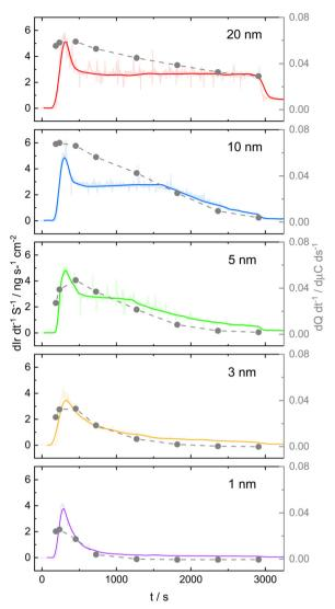
Correlation between Ir dissolution and HIROF growth. Left y-axis: Dissolution rate; right y-axis: first derivative of total anodic charge from Fig. 2(c)
