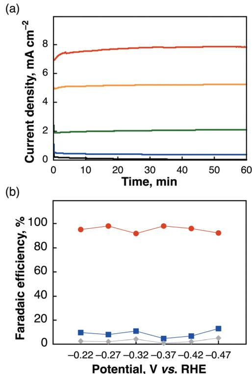
Fig. 2 (a) Chronoamperograms over a [**Mes-IrPPh2**] cathode and a Pt anode for 1 h with several bias voltages [ $-0.07$  V (black),  $-0.17$  V (blue),  $-0.27$  V (green),  $-0.37$  V (orange),  $-0.47$  V (red)] and (b) FEs of the products [HCOO<sup>-</sup> (red), CO (blue), H<sub>2</sub> (gray)] obtained during the electrocatalytic CO<sub>2</sub> reduction using a [**Mes-IrPPh2**] electrode in a solution of CO<sub>2</sub>-saturated 0.5 M KHCO<sub>3</sub>.
