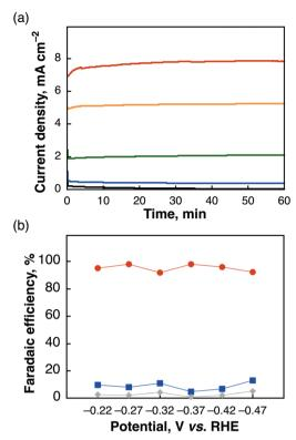
Fig. 2 (a) Chronoamperograms over a [Mes-IrPPh2] cathode and a Pt anode for 1 h with several bias voltages [-0.07 V (black), -0.17 V (blue), -0.27 V (green), -0.37 (orange), -0.47 V (red)] and (b) FEs of the products [HCOO $^-$  (red), CO (blue), H $_2$  (gray)] obtained during the electrocatalytic CO $_2$  reduction using a [Mes-IrPPh2] electrode in a solution of CO $_2$ -saturated 0.5 M KHCO $_3$ .
