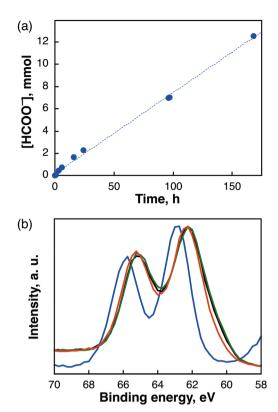
**Fig. 3** (a) Time course plots of the HCOO $^-$  obtained during the electrocatalytic CO $_2$  reduction at -0.27 V vs. RHE using a [**Mes-IrPPh2**] cathode and a Pt anode in a solution of CO $_2$ -saturated 0.5 M KHCO $_3$ . (b) Ir 4f XPS spectra of a [**Mes-IrPPh2**] electrode [before (blue) and after electrolysis for 3 h (black), 15 h (green), 72 h (red)].
