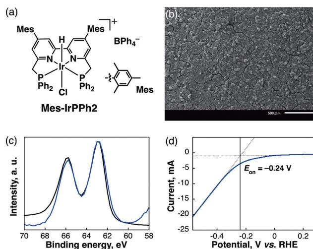
Fig. 1 (a) Chemical structure of **Mes-IrPPh2**. (b) A SEM image of the [**Mes-IrPPh2**] electrode. Scale bar is  $500 \mu\text{m}$ . (c) Ir 4f XPS spectra of the [**Mes-IrPPh2**] (blue line) electrode and  $\text{Ir}^{\text{III}}\text{Cl}_3 \cdot \text{H}_2\text{O}$  (black line) as a reference. (d) LSV for the [**Mes-IrPPh2**] electrocatalyst in a  $\text{CO}_2$ -saturated  $0.5 \text{ M KHCO}_3$  solution.
