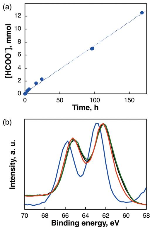
**Fig. 3** (a) Time course plots of the  $\text{HCOO}^-$  obtained during the electrocatalytic  $\text{CO}_2$  reduction at  $-0.27$  V vs. RHE using a [Mes-IrPPh<sub>2</sub>] cathode and a Pt anode in a solution of  $\text{CO}_2$ -saturated 0.5 M  $\text{KHCO}_3$ . (b) Ir 4f XPS spectra of a [Mes-IrPPh<sub>2</sub>] electrode [before (blue) and after electrolysis for 3 h (black), 15 h (green), 72 h (red)].
