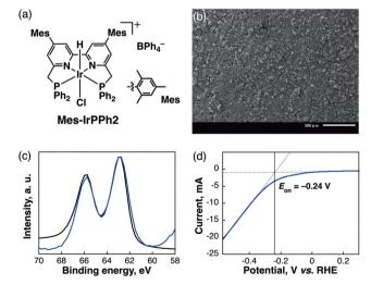
Fig. 1 (a) Chemical structure of Mes-IrPPh2. (b) A SEM image of the [Mes-IrPPh2] electrode. Scale bar is 500  $\mu$ m. (c) Ir 4f XPS spectra of the [Mes-IrPPh2] (blue line) electrode and Ir  $^{II}$ Cl $_3$ ·H $_2$ O (black line) as a reference. (d) LSV for the [Mes-IrPPh2] electrocatalyst in a CO $_2$ -saturated 0.5 M KHCO $_3$  solution.
