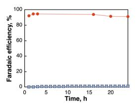
Fig. 4 Time course plots of the product [HCOO $^-$  (red), CO (blue), H $_2$  (gray)] obtained during the CO $_2$  electrochemical reduction using a [Mes-IrPPh2] cathode and Fe/Ni–Ni foam anode under simulated solar light irradiation.
