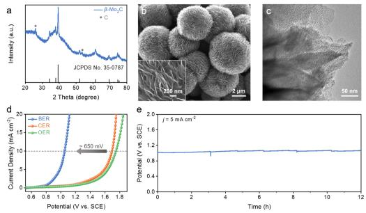
Fig. 2 Structural characterizations and electrocatalytic BER performance of Mo<sub>2</sub>C NF. (a) XRD pattern. (b) SEM and (c) TEM image of Mo<sub>2</sub>C NF. (d) Polarization curves of the BER, CER, and OER on Mo<sub>2</sub>C NF in 0.1 M KBr, 0.1 M KCl, and 0.1 M K<sub>2</sub>SO<sub>4</sub> solution. (e) Chronopotentiometric curve of the BER on Mo<sub>2</sub>C NF at 5 mA cm<sup>-2</sup> in 0.1 M KBr solution
