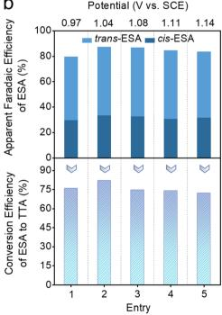
Fig. 4 Hydrolysis conversion of ESA to TTA. (a) Reaction mechanism from ESA to TTA. (b) Conversion efficiency of five ESA samples obtained from bromine-mediated conversion at different working potentials.
