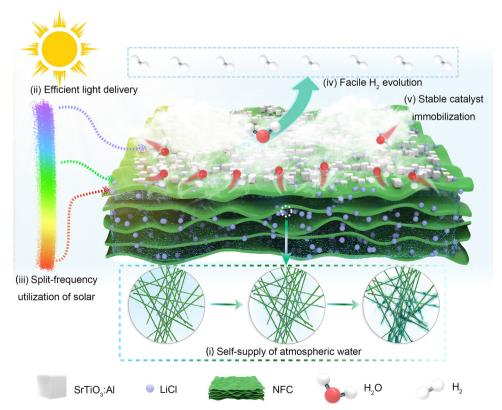
Fig. 1 Schematic illustration of the NLS gel and its application in solar-powered in situ H<sub>2</sub> production from air. (i) Self-supply of atmospheric water, i.e., absorption of water vapor from the air, liquefaction, liquid water transport and storage, (ii) efficient light delivery, (iii) complementary utilization of solar energy in split frequency, (iv) facile H2 evolution, and (v) stable catalyst immobilization.
