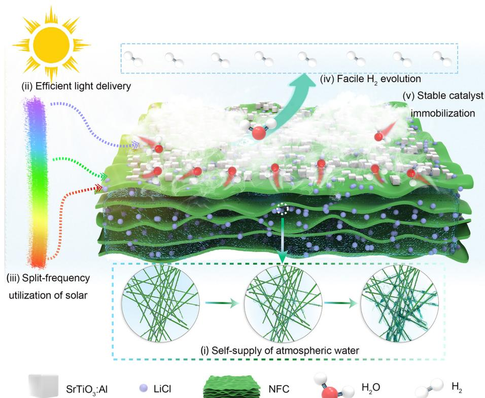
**Fig. 1** Schematic illustration of the NLS gel and its application in solar-powered *in situ* H<sub>2</sub> production from air. (i) Self-supply of atmospheric water, *i.e.*, absorption of water vapor from the air, liquefaction, liquid water transport and storage, (ii) efficient light delivery, (iii) complementary utilization of solar energy in split frequency, (iv) facile H<sub>2</sub> evolution, and (v) stable catalyst immobilization.
