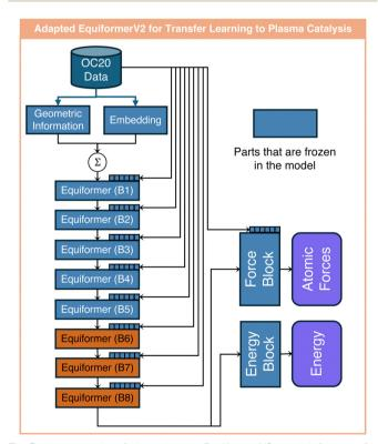
Fig. 3 An example of the adapted EquiformerV2 model for transfer learning to plasma catalysis. The layers up to and including the fifth Equiformer block (B5) and the force and energy blocks are frozen. The atom embeddings are frozen, including in the Equiformer blocks B6-B8. However, the proton embeddings of all layers are unfrozen and are updated during transfer learning, initialized from hydrogen embeddings of the pre-trained model.
