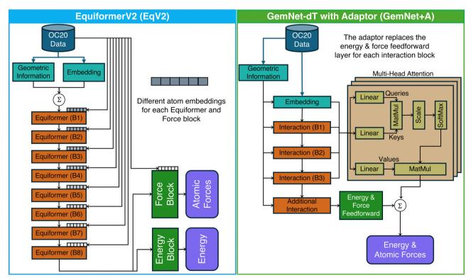
Fig. 2 Architectures of the two graph neural network models, pre-trained using the OC20 dataset for thermal catalysis.<sup>28</sup> The left is the EquiformerV2 architecture with eight Equiformer blocks. 40 The right is the GemNet-dT architecture 39 with a multi-head attention adaptor for improved transfer learning.<sup>32</sup> The number of additional interaction blocks is set to one.
