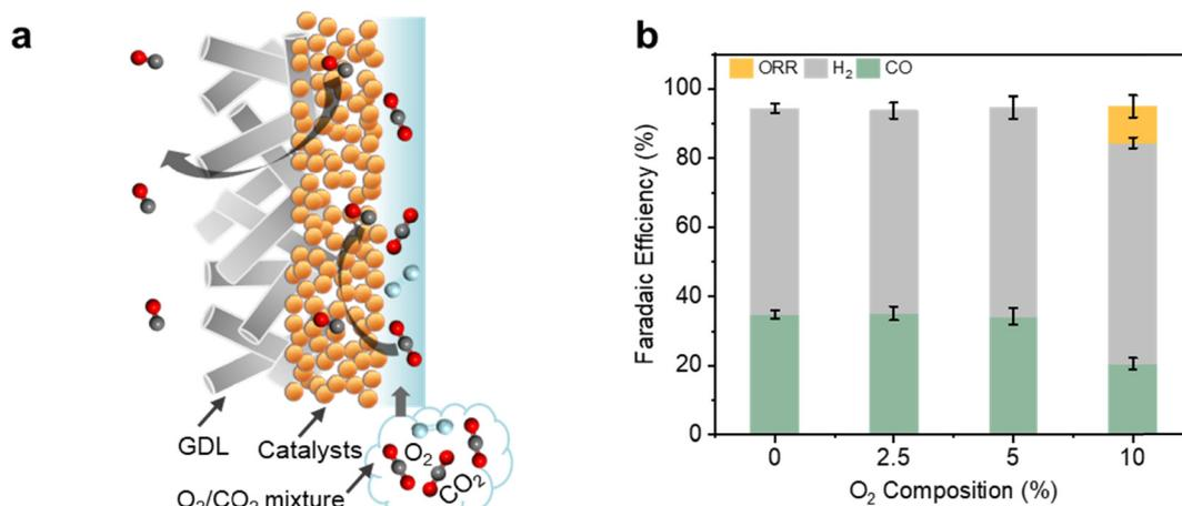
**Fig. 6** Oxygen-tolerant CO<sub>2</sub>R with the reversed GDE. (a) Schematic showing electrolysis with feedstock containing O<sub>2</sub> impurities. (b) CO<sub>2</sub>R product FE obtained with different O<sub>2</sub> impurity compositions. In all cases, a constant current density of 80 mA cm<sup>-2</sup> was applied with 1 M KHCO<sub>3</sub> as the electrolyte. We calculated the ORR FE by assuming that all missing FE can be entirely attributed to ORR.
