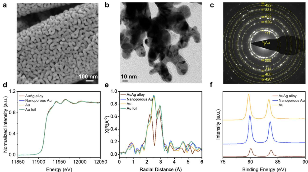
Fig. 4 Structure characterization of nanoporous Au. (a) SEM images of nanoporous Au. (b) Bright-field TEM images of nanoporous Au. (c) Selected-area electron diffraction (SAED) patterns of nanoporous Au. (d) Au  $L_3$ -edge X-ray absorption near edge spectroscopy (XANES) of Au based catalyst. (e) Au  $L_3$ -edge Fourier-transformed (FT)  $k^2$ -weighted  $\chi(k)$  functions of Au based catalysts. (f) Au 4f X-ray photoelectron spectroscopy (XPS) spectra of the different Au based samples.
