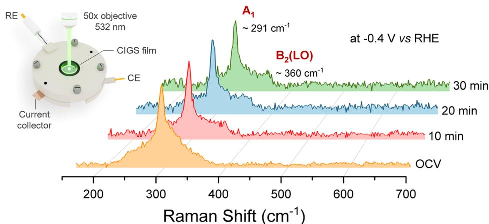
**Fig. 4** *Operando* Raman spectra showing the time evolution of the CIGS photocathode under CO<sub>2</sub>R operation at  $-0.4 \text{ V vs. RHE}$  in CO<sub>2</sub>-saturated 0.1 M KHCO<sub>3</sub>.
