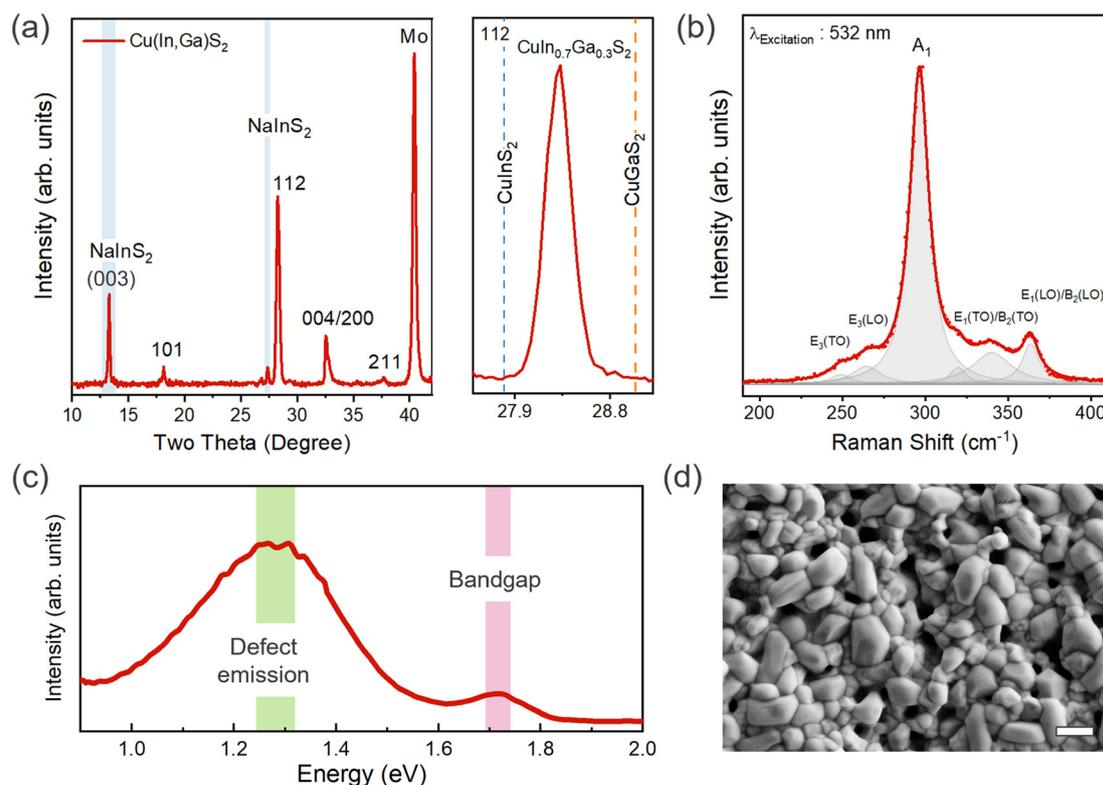
**Fig. 1** (a) XRD diffractograms and (b) Raman spectrum of the CIGS thin film, (c) PL from a wide spectral range showing a bandgap at  $\sim 1.77\text{ eV}$  and broad emission at  $\sim 1.3\text{ eV}$  corresponding to deep defect(s), and (d) SEM image of the CIGS thin film showing the surface morphology. Scale bar:  $1\text{ }\mu\text{m}$ .
