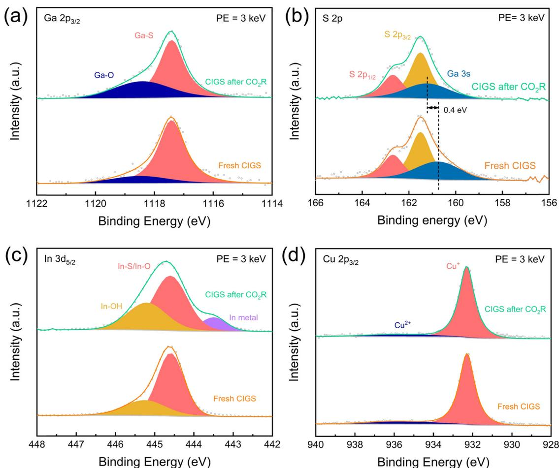
Fig. 5 Deconvoluted XPS spectra on the CIGS before and after 80 min of  $\text{CO}_2\text{R}$  operation. (a) Ga  $2p_{3/2}$ , (b) S 2p, (c) In  $3d_{5/2}$ , and (d) Cu  $2p_{3/2}$  photoelectron peaks and curve fitting results (solid color area) of the fresh CIGS (bottom) and CIGS after  $\text{CO}_2\text{R}$  (upper), respectively (photon energy = 3 keV).
