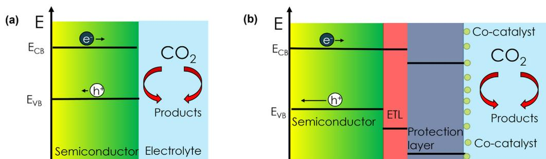
**Scheme 1** (a) Configuration (1) direct semiconductor/electrolyte for PEC CO<sub>2</sub>R. (b) Configuration (2) buried semiconductor for PEC CO<sub>2</sub>R. (Band bending is omitted for simplicity).
