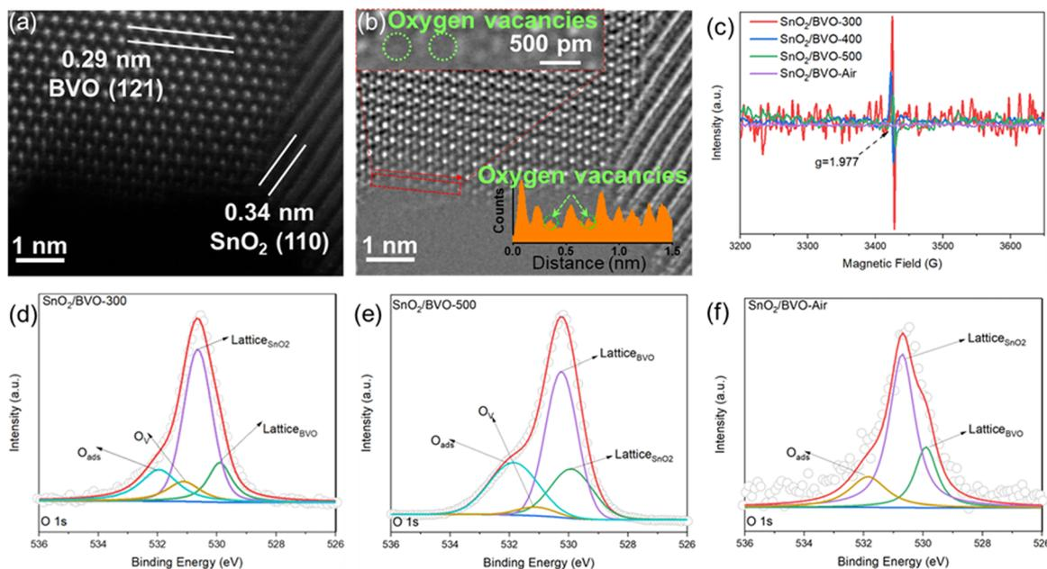
Fig. 2 (a) and (b) HAADF and iDPC images of the SnO<sub>2</sub>/BVO-400 sample. (c) EPR spectra of BVO-300, BVO-400, BVO-500, and BVO-Air. (d)–(f) High-resolution O 1s spectra of SnO<sub>2</sub>/BVO-300, SnO<sub>2</sub>/BVO-500, and SnO<sub>2</sub>/BVO-Air.
