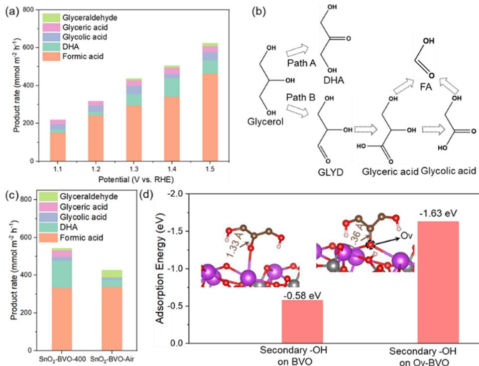
Fig. 5 (a) PEC glycerol oxidation product rate of the SnO<sub>2</sub>/BVO-400 photoanode at different bias potentials. (b) Illustration of the typical glycerol oxidation pathway. (c) PEC glycerol oxidation product rates of SnO<sub>2</sub>/BVO-400 and SnO<sub>2</sub>/BVO-Air at a bias of 1.4 V vs. RHE. (d) DFT-optimized structures of the secondary OH<sup>-</sup> group adsorbed on general BVO and Ov-BVO.
