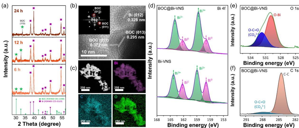
Fig. 3 Phase transition of Bi-VNS. (a) XRD patterns of BOC@Bi-VNS formed after different CO<sub>2</sub>RR times. (b) HRTEM image and FFT pattern (inset), and (c) HAADF-STEM image and EDS elemental mapping of BOC@Bi-VNS after 24 h of the CO<sub>2</sub>RR. (d) High resolution XPS Bi 4f spectra of BOC@Bi-VNS and Bi-VNS. (e) O 1s, and (f) C 1s spectra of BOC@Bi-VNS.
