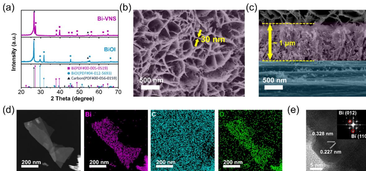
**Fig. 1** Characterization of Bi-VNS. (a) XRD patterns of BiOI and Bi-VNS (bismuth vertical nanosheet). SEM images of Bi-VNS in (b) top view, and (c) cross-sectional view. For visual clarity, Bi-VNS and carbon paper are colored purple and blue, respectively. (d) HAADF-STEM image and EDS elemental mapping of Bi-VNS. (e) HRTEM image and FFT pattern (inset) of Bi-VNS.
