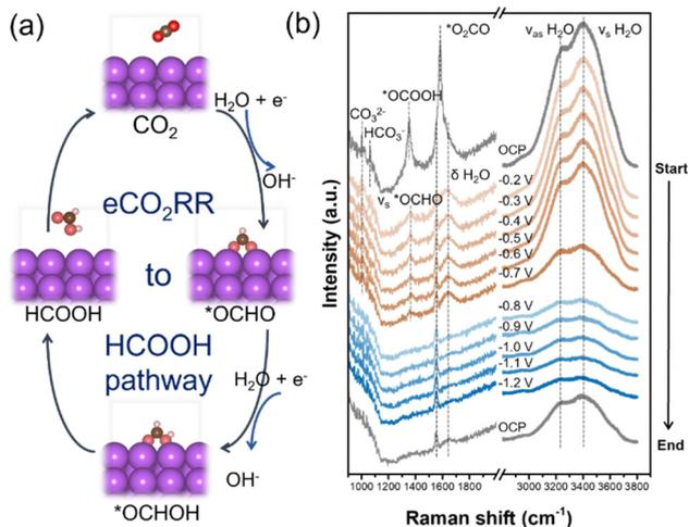
Fig. 4 *In situ* Raman spectroscopy (a) schematic of the electrochemical CO<sub>2</sub>RR (eCO<sub>2</sub>RR) to the formic acid pathway and (b) *in situ* Raman spectra in CO<sub>2</sub>-saturated 0.2 M KHCO<sub>3</sub> electrolyte solution. The Raman spectra were recorded stepwise starting from OCP to  $-1.2 V_{RHE}$  and back to OCP.
