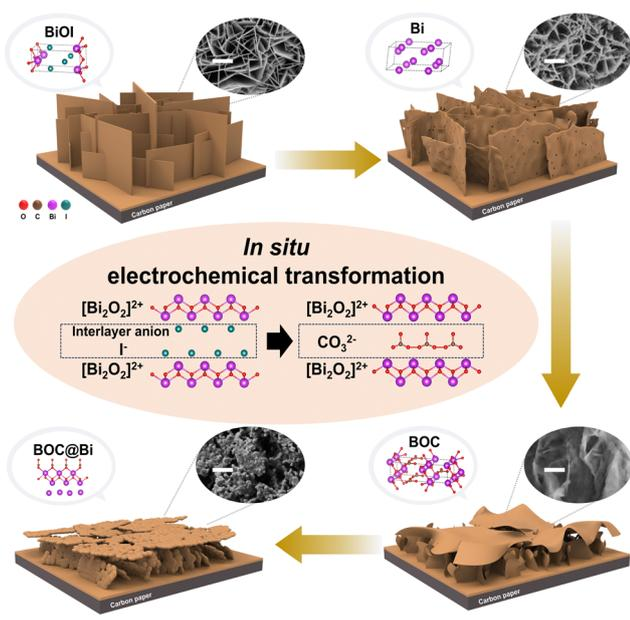
Fig. 6 Schematic illustration of the *in situ* transformation of the BiOI-derived cathode. The morphology and phase of BiOI vertical nanosheets change significantly during the electrochemical reduction reaction. The similarity between the layered structures of BiOI and BOC enables the *in situ* transformation of BiOI into Bi, and then BOC.
