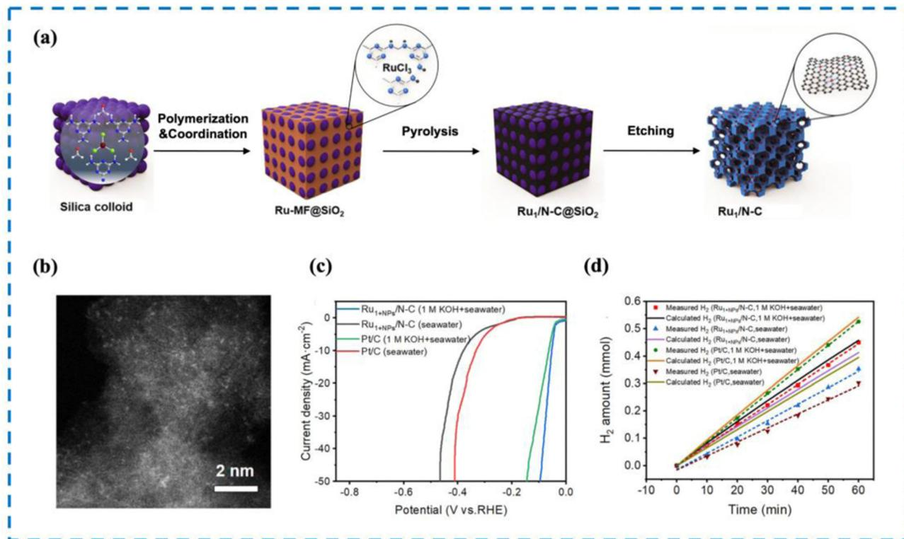
Fig. 10 Synthesis, HAADF-STEM and HER performance of  $\text{Ru}_{1+\text{NPs}}/\text{N}-\text{C}$ . (a) Synthesis of  $\text{Ru}_{1+\text{NPs}}/\text{N}-\text{C}$ . (b) HAADF-STEM image. (c) LSV curve in seawater and 1 M KOH. (d) FE in seawater and 1 M KOH.<sup>188</sup> This figure has been adapted/reproduced from ref. 188 with permission from American Chemical Society, copyright©2022, American Chemical Society.
