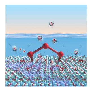
Fig. 4 Schematic diagram of the "five-membered cycle" mechanism during the EOP process presented by our group.
