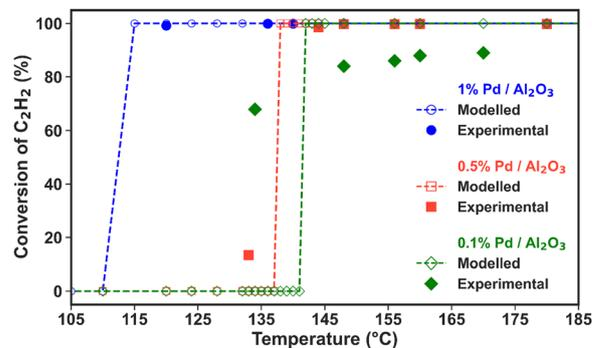
Fig. 3 Experimental and modelled  $C_2H_2$  conversion as a function of temperature (average temperature measured in the catalyst bed and assumed to be identical for solid and gas phases) for the three  $Pd/Al_2O_3$  catalysts (see the legend). The number of experimental data points (solid markers) is different for each catalyst.
