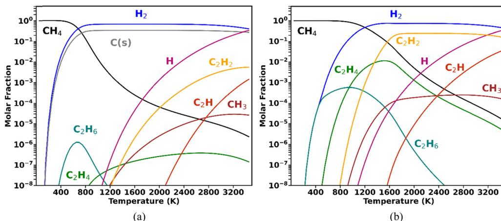
Fig. 1 Gas-phase equilibrium composition at 1 bar, initiated with 1 mole of CH<sub>4</sub>, under two assumptions: (a) solid carbon is formed in equilibrium with the gas phase, or (b) there is no formation of a solid phase.
