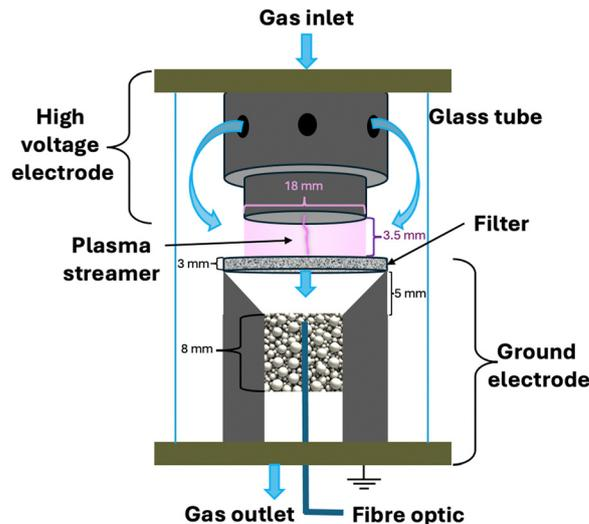
Fig. 2 Schematic of the plate-to-plate plasma reactor with a post-plasma catalytic bed for hydrogenation. Experiments carried out with 100 sccm CH<sub>4</sub> and 100 sccm H<sub>2</sub>, with three bursts at 10 kHz, 3000 p s<sup>-1</sup>, 50% voltage amplitude. The catalytic bed is composed of 200 mg Pd/Al<sub>2</sub>O<sub>3</sub> and 800 mg Al<sub>2</sub>O<sub>3</sub>.
