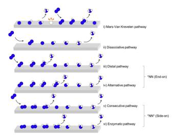
Fig. 2 Direct electrocatalytic N<sub>2</sub> reduction. Electrocatalytic NRR reduction pathways, (i) Mars-van Krevelen (MvK), (ii) dissociative (iii) distal and (iv) alternative pathway initiated with \*NN end-on adsorption, (v) consecutive and (vi) enzymatic initiated with \*NN side-on adsorption.
