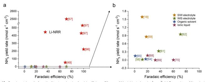
Fig. 10 Experimental results from the literature showing faradaic efficiency (%) versus NH<sub>3</sub> yield rate (nmol s<sup>-1</sup> cm<sup>-2</sup>). (a) Comparison of N<sub>2</sub> reduction performance for both direct eNRR and Li-NRR mechanisms. (b) Enlarged view comparing N2 reduction in the direct eNRR mechanism through various electrolyte engineering approaches.
