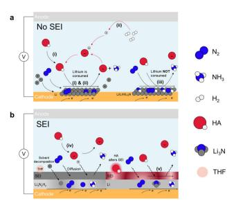
Fig. 3 Indirect Li-NRR. Schematic for lithium-mediated NRR with (a) no SEI formed and (b) SEI formed. Five potential mechanisms are summarized.  $^{48}$  These include lithium cycling with (i) proton source from the electrolyte<sup>50</sup> and (ii) proton shuttle model in which proton is from H<sub>2</sub> oxidation.49 (iii) Electro-driven Li-NRR where lithium only provides the electron. 46 SEI diffusion model for (iv) non-reactive SEI, 47 and (v) adjusted permeable SEI layer through HA.51
