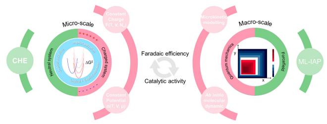
Fig. 11 Schematic illustration of computation techniques for electrolyte engineering, spanning from microscopic descriptors employing quantum-level based calculations that include solvation and electrode potential effects, to macroscopic kinetic strategies, bridging the gap for practical electrochemical performances
