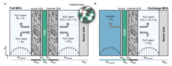
Fig. 1 Schematic representations of the computational domains used in this work. The feed flows in the y-direction whereby the serpentine motion is neglected for simplicity. (a) Full MEA configuration is fed with a gaseous feed at both anode and cathode. (b) Exchange MEA configuration is fed liquid electrolyte at the anode side. The cathode compartment is fed humidified CO<sub>2</sub>. Details regarding dimensions are provided in the ESI,† Table S8.
