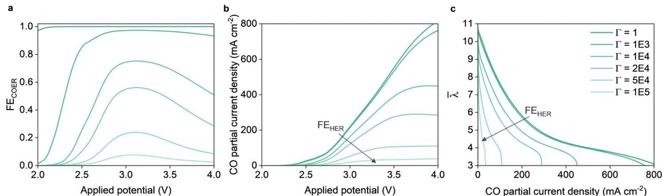
**Fig. 7** Electrochemical performance of a full MEA simulated with increased HER kinetics. (a) Faradaic efficiency of the carbon monoxide evolution reaction at various potential for different degrees of increased HER kinetics ( $\Gamma$ ). (b) Polarization curves and (c) average membrane water content for the various degrees of HER amplification.
