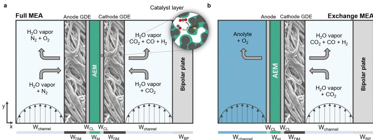
**Fig. 1** Schematic representations of the computational domains used in this work. The feed flows in the *y*-direction whereby the serpentine motion is neglected for simplicity. (a) Full MEA configuration is fed with a gaseous feed at both anode and cathode. (b) Exchange MEA configuration is fed liquid electrolyte at the anode side. The cathode compartment is fed humidified CO<sub>2</sub>. Details regarding dimensions are provided in the ESI,<sup>†</sup> Table S8.
