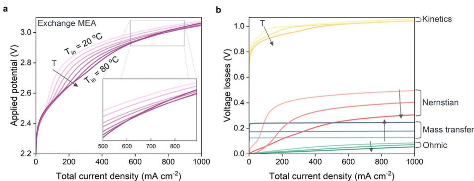
Fig. 6 (a) Polarization curves for the simulated exchange MEA at various operating temperatures ranging from 20 to  $80 \text{ }^\circ\text{C}$  with increments of 10 degrees. (b) Voltage breakdown analysis of the major contributions to the voltage losses for the simulated exchange MEA at operating temperatures of 20, 50 and  $80 \text{ }^\circ\text{C}$ .
