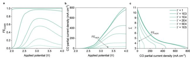
Fig. 7 Electrochemical performance of a full MEA simulated with increased HER kinetics. (a) Faradaic efficiency of the carbon monoxide evolution reaction at various potential for different degrees of increased HER kinetics ( $\Gamma$ ). (b) Polarization curves and (c) average membrane water content for the various degrees of HER amplification.
