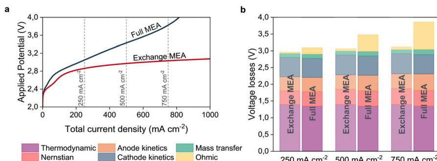
Fig. 4 Comparison of the electrochemical performance of the exchange- and full MEA configurations for  $y = 0$  operated at ambient conditions. (a) Polarization curves for the two configurations reveal a significantly higher energy requirement for the full MEA. (b) Breakdown of the voltage losses for total current densities of 250, 500 and 750 [mA cm<sup>-2</sup>] which are indicated in figure a with vertical lines.
