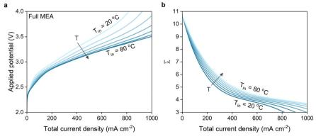
Fig. 5 (a) Polarization curves for the simulated full MEA at various operating temperatures ranging from 20 to 80 °C with increments of 10 degrees for y = 0. (b) Average membrane water content versus the total current density for the same case.
