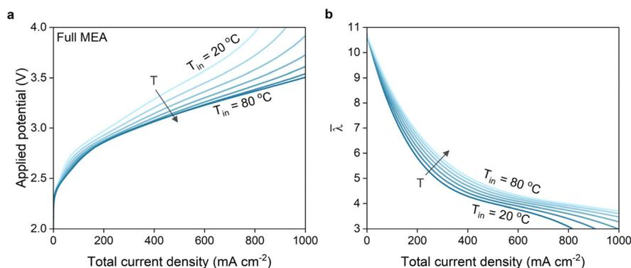
Fig. 5 (a) Polarization curves for the simulated full MEA at various operating temperatures ranging from 20 to 80 °C with increments of 10 degrees for  $y = 0$ . (b) Average membrane water content versus the total current density for the same case.
