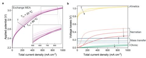
Fig. 6 (a) Polarization curves for the simulated exchange MEA at various operating temperatures ranging from 20 to 80 °C with increments of 10 degrees. (b) Voltage breakdown analysis of the major contributions to the voltage losses for the simulated exchange MEA at operating temperatures of 20, 50 and 80 °C.
