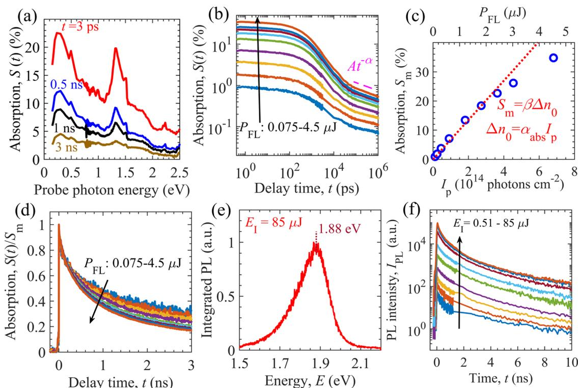
Fig. 2 Absorption and photoluminescence spectroscopies of the GTOS photocatalyst. (a) TDR signal  $S(t)$  spectra. (b)  $S(t)$  kinetics at a probe photon energy of 0.24 eV. (c) Maximum absorption signal  $S_m$  (at  $t \sim 0.4$  ps) as functions of the pump fluence intensity  $P_{FL}$  and pump photon density  $I_p$ . (d) Normalized absorption signal  $S(t)/S_m$  decays. (e) Integrated photoluminescence spectrum. (f) TPL signal  $I_{PL}$  decays at various excitation intensities  $E_I$ .
