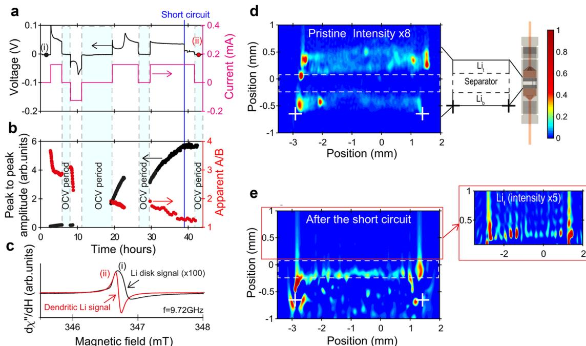
**Fig. 9** (a)–(e) *In situ* detection (EPR spectrum) and localization (EPR images) of dendritic Li. Reprinted with permission from ref. 46 Copyright 2021, Springer Nature.
