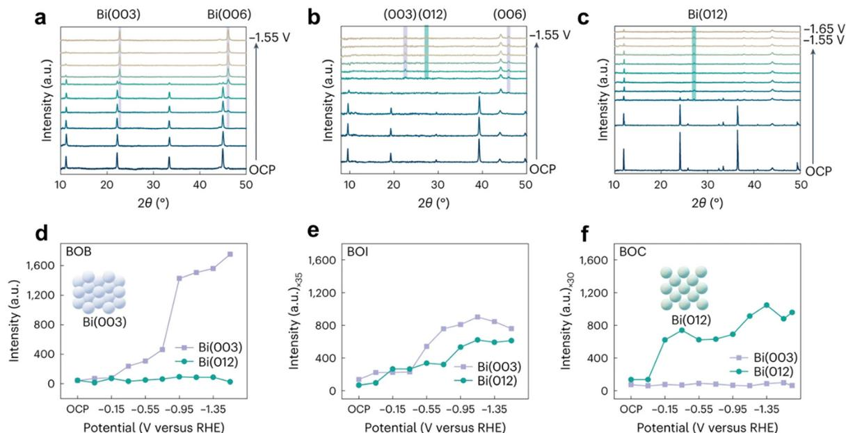
Fig. 5 *In situ* XRD of (a) BOB, (b) BOI and (c) BOC. Diffraction intensity of Bi(003) and Bi(012) facets as a function of the reaction time of BOB (d), BOI (e) and BOC (f) in CO<sub>2</sub> saturated 0.1 M KHCO<sub>3</sub> solution. The purple and green shaded areas give the expected diffraction angles for the Bi(003) and Bi(006) reflections and Bi(012) reflections, respectively. Reprinted with permission from ref. 25 Copyright 2023, Springer Nature.
