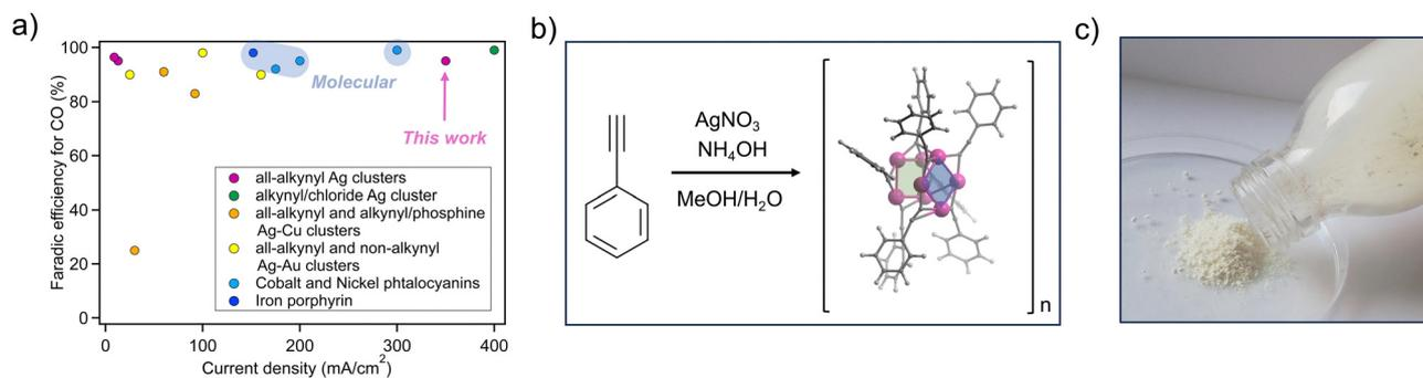
**Fig. 1** (a) Graph depicting the faradaic efficiency for CO vs. current density of state-of-the-art silver-based clusters catalysts, in comparison with the best performing molecular catalysts; (b) general scheme of silver acetylide’s synthesis with a representation of an asymmetric unit of the cluster fragment established by electron diffraction showing two Ag<sub>4</sub> clusters subunits; (c) picture of the catalysts powder used for structure resolution by 3D-ED.
