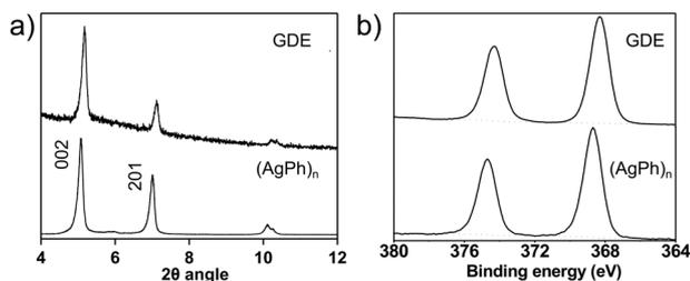
Fig. 4 (a) Powder diffractograms of the pristine catalyst powder (AgPh)<sub>n</sub> and of the GDE after catalyst deposition; (b) XPS spectra in the Ag 3d emission region of the pristine catalyst powder and GDE after catalyst deposition.
