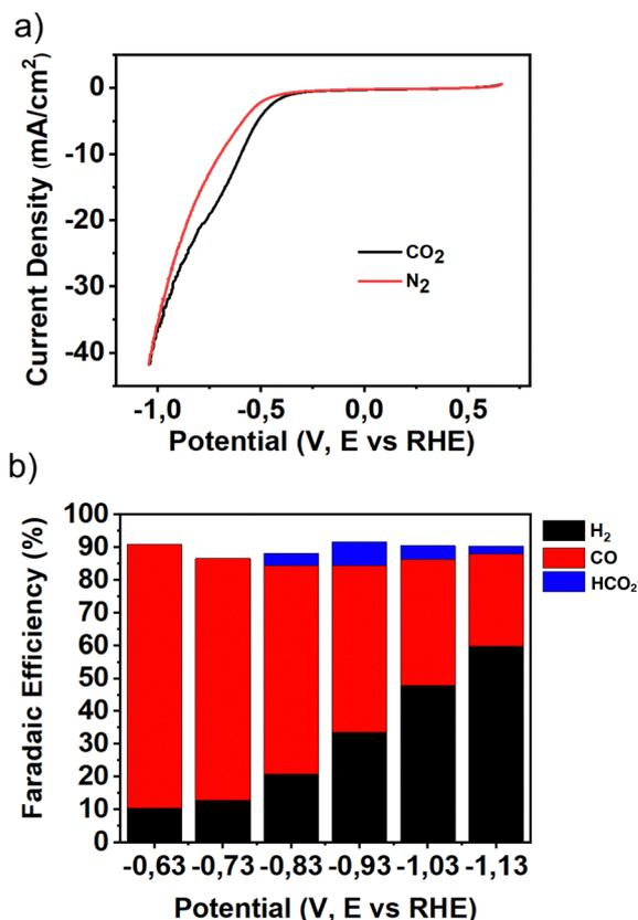
Fig. 5 (a) Linear sweep voltammetry plot of (AgPh)<sub>n</sub> carried out in KHCO<sub>3</sub> (0.5 M) under an N<sub>2</sub> or CO<sub>2</sub> saturated solution; (b) Faradaic efficiencies for H<sub>2</sub>, CO and formate extracted from chronoamperometry experiments carried out in incremental potential values and sampled after 30 min of reaction.
