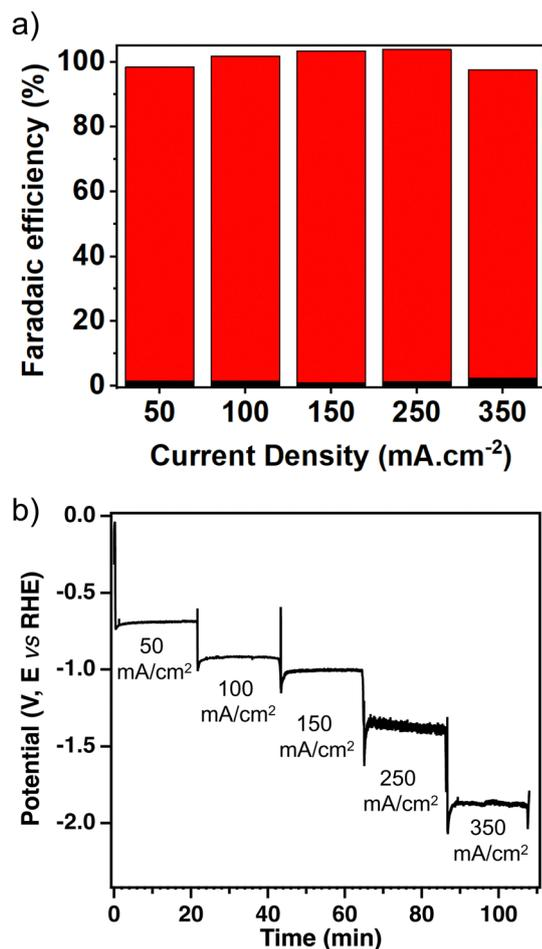
Fig. 6 (a) Faradaic efficiency of (AgPh)<sub>n</sub> under CO<sub>2</sub> reduction conditions in a flow cell electrolyser (KHCO<sub>3</sub> (1 M) as catholyte and anolyte); (b) Cathode potential of the best-performing GDE (vs. RHE with *iR* drop correction).
