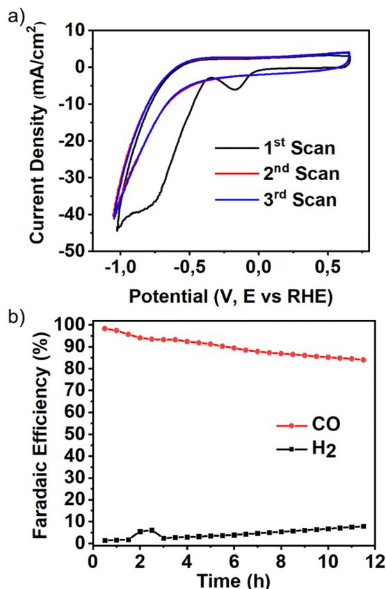
Fig. 7 (a) Cyclic voltammetry of Ag showing three consecutive cycles in the 0 to -1.4 V range (vs. RHE); (b) faradaic efficiency evolution over time at 100 mA cm<sup>-2</sup>.
