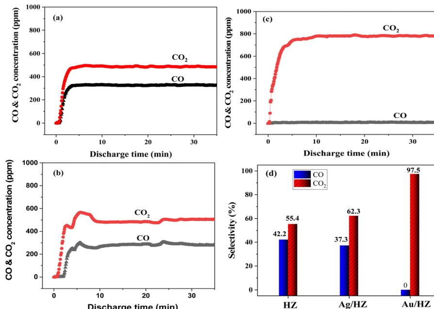
Fig. 6 CO and CO<sub>2</sub> concentrations of gaseous C<sub>7</sub>H<sub>8</sub> oxidation in dry simulated air plasma over (a) HZ, (b) Ag/HZ (1.2 wt% Ag), and (c) Au/HZ (0.6 wt% Au), and (d) their corresponding CO<sub>x</sub> selectivities. Conditions: 100 mL min<sup>-1</sup> of simulated air with 115 ppm C<sub>7</sub>H<sub>8</sub>, P<sub>in</sub> = 7.0 W.
