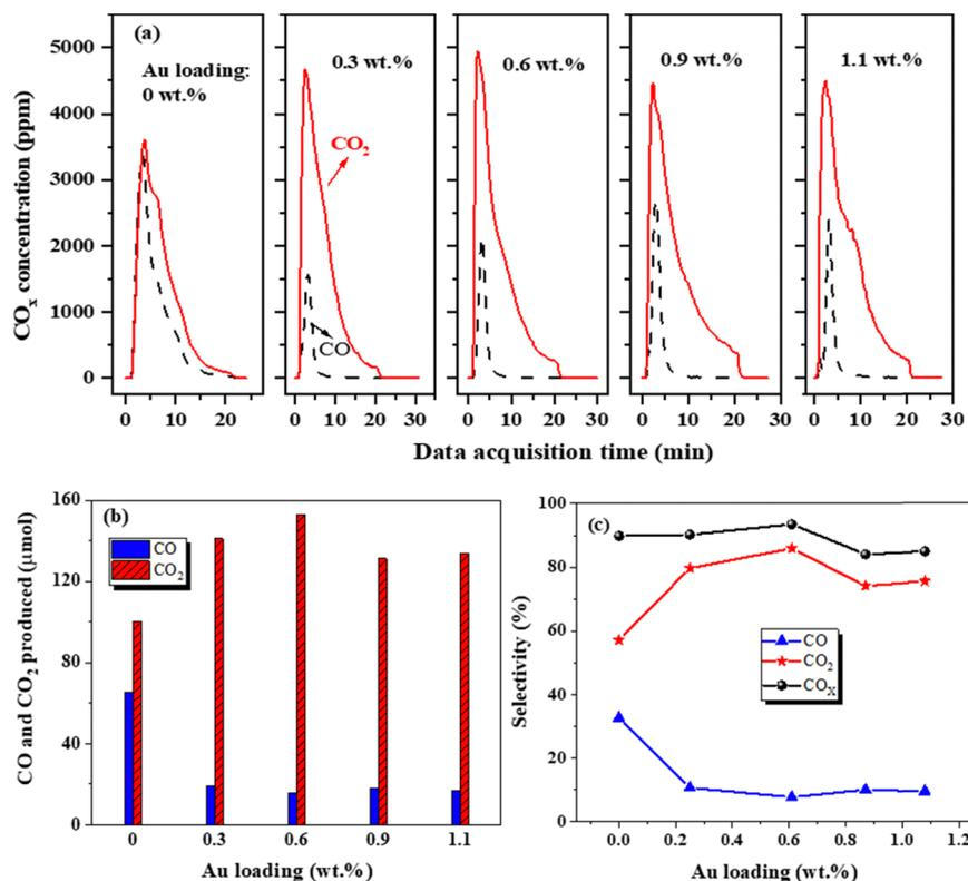
Fig. 4 Effect of Au loading on (a)  $CO_x$  concentration, (b) the amount of  $CO_x$  produced, and (c)  $CO_x$  selectivities in plasma oxidation of adsorbed  $C_7H_8$  on Au/HZ. Conditions:  $n_{C_7H_8}^0 = 25.2 \mu\text{mol}$ ,  $P_{in} = 7.0 \text{ W}$ ,  $t_{dis} = 20 \text{ min}$ ,  $100 \text{ mL min}^{-1}$  of dry simulated air.
