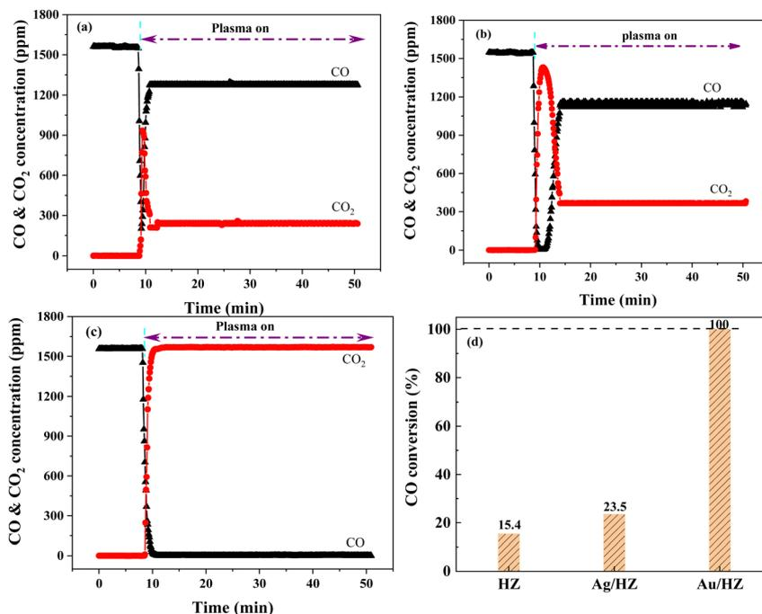
Fig. 7 CO and CO<sub>2</sub> concentrations of CO oxidation in dry simulated air plasma over (a) HZ, (b) Ag/HZ (1.2 wt% Ag), and (c) Au/HZ (0.6 wt% Au), and (d) the corresponding CO conversion over different catalysts. Conditions: 100 mL min<sup>-1</sup> of simulated air with 1555 ppm CO, m<sub>cat</sub> = 0.20 g, P<sub>in</sub> = 7.0 W.
