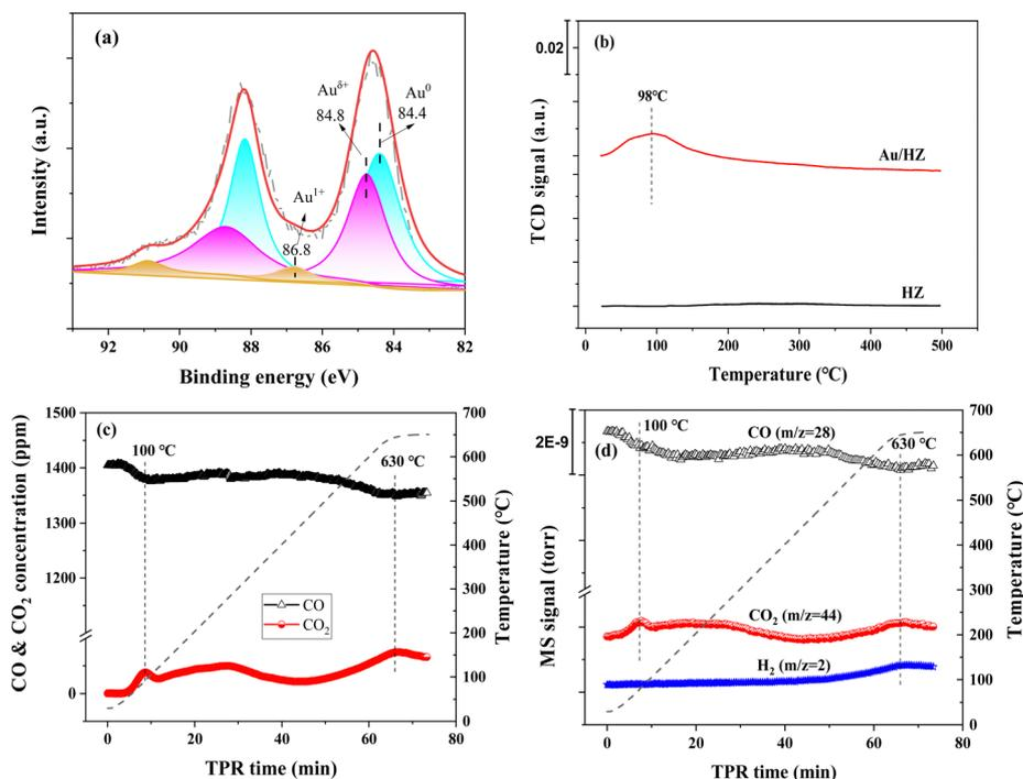
Fig. 2 (a) XPS spectrum of Au 4f in Au/HZ; (b) H<sub>2</sub>-TPR profiles of Au/HZ and HZ; and (c) CO and CO<sub>2</sub> concentrations and (d) MS signals of CO, CO<sub>2</sub> and H<sub>2</sub> in CO-TPR tests over Au/HZ (0.6 wt% Au). H<sub>2</sub>-TPR conditions: 30 mL min<sup>-1</sup> of 5% H<sub>2</sub>/Ar, 0.20 g Au/HZ. CO-TPR conditions: 100 mL min<sup>-1</sup> of 1400 ppm CO/He.
