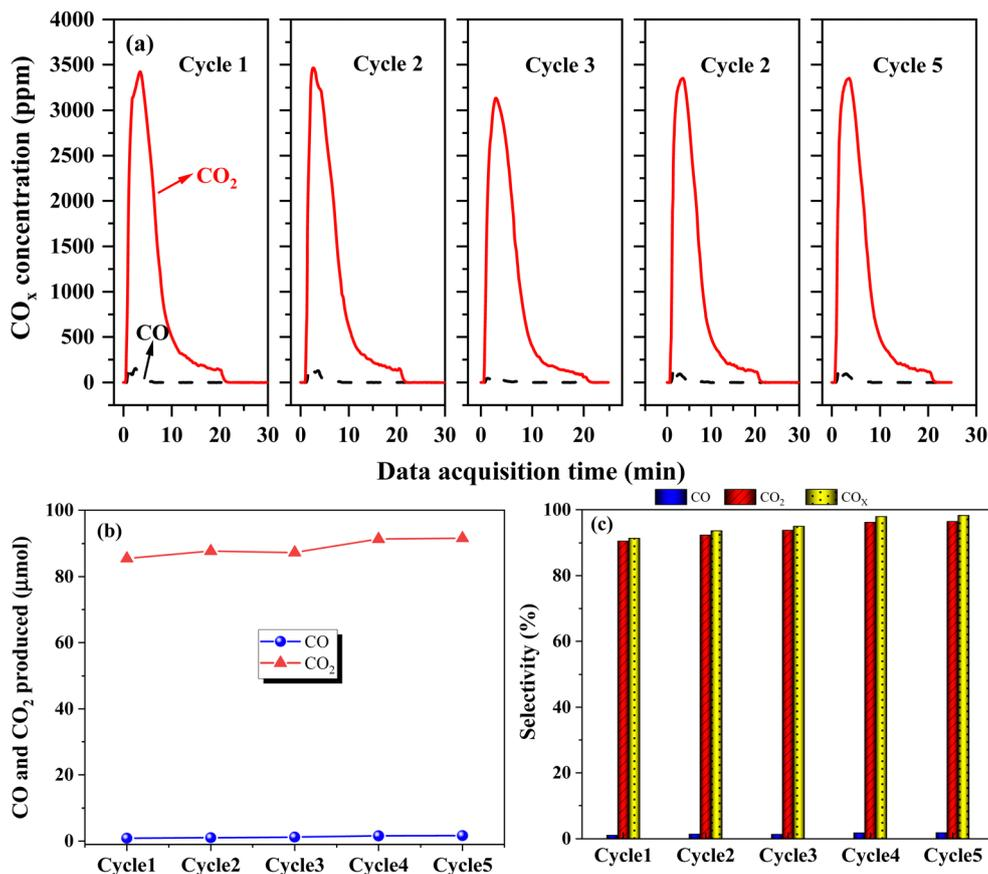
Fig. 5 (a) CO<sub>x</sub> concentration, (b) amounts of CO and CO<sub>2</sub> produced, and (c) CO, CO<sub>2</sub>, and CO<sub>x</sub> selectivities of five cycles of C<sub>7</sub>H<sub>8</sub> CSD oxidation over the Au/HZ catalyst. Conditions:  $n_{\text{C}_7\text{H}_8}^0 = 13.5 \mu\text{mol}$ ,  $P_{\text{in}} = 7.0 \text{ W}$ ,  $t_{\text{dis}} = 20 \text{ min}$ ,  $100 \text{ mL min}^{-1}$  of dry simulated air.
