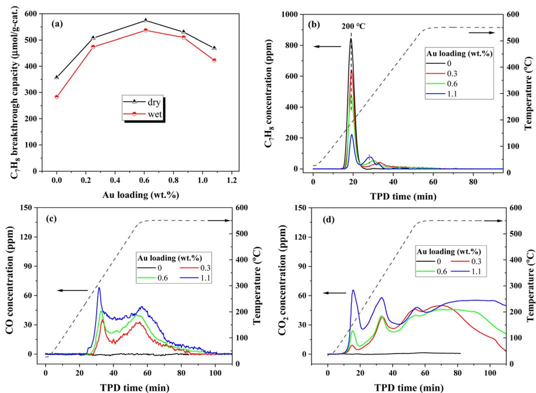
Fig. 3 Effect of Au loading on (a) C<sub>7</sub>H<sub>8</sub> breakthrough capacity under dry and wet conditions; (b) C<sub>7</sub>H<sub>8</sub> concentration, (c) CO concentration, and (d) CO<sub>2</sub> concentration in TPD tests. Adsorption conditions: 100 mL min<sup>-1</sup> of dry or wet (RH = 66%, 20 °C) simulated air with C<sub>7</sub>H<sub>8</sub>; TPD conditions:  $n_{C_7H_8}^0 = 13.5 \mu\text{mol}$ , 100 mL min<sup>-1</sup> of Ar.
