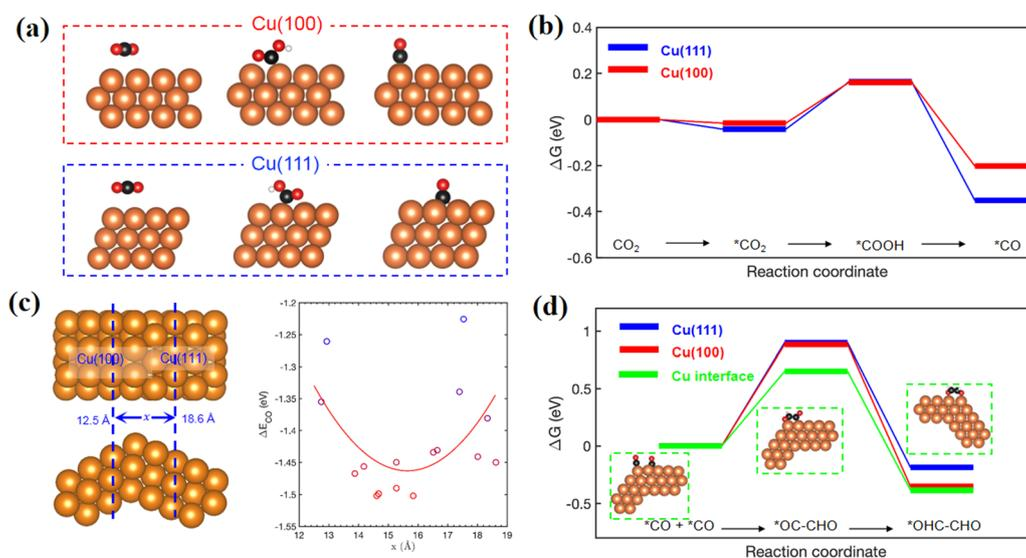
Fig. 5 DFT calculations. (a) DFT models of Cu with different facets. (b) Free energy diagram for CO<sub>2</sub> reduction into \*CO on the Cu(111) and (100) surfaces at  $U = 0$  V. (c) CO adsorption energy in the vicinity of the Cu(111)/(100) interface. (d) Free energy diagram for reductive CO-CO coupling on Cu(111), Cu(100) and Cu(111)/(100) interface at  $U = 0$  V.
