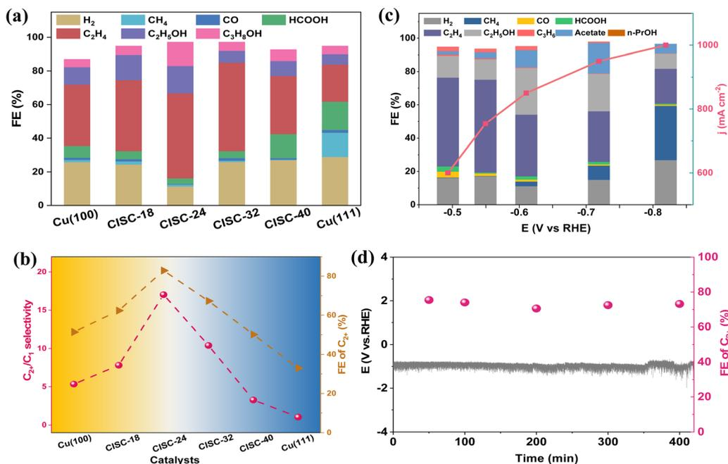
Fig. 3 CO<sub>2</sub>RR performance. (a) Faradaic efficiency of various products at  $-1.1$  V in the H-type cell; (b) faradaic efficiency of C<sub>2+</sub> and product ratio of C<sub>2+</sub>/C<sub>1</sub> on different types of Cu catalysts at  $-1.1$  V; (c) faradaic efficiency of CISC-24 at various potentials in a flow cell. (d) Long-term CO<sub>2</sub>RR stability test of Cu-24 in 1 M KHCO<sub>3</sub> electrolyte at a constant current density of 300 mA cm<sup>-2</sup>.
