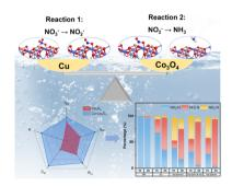
Fabrication of dual-sited Cu doped Co<sub>3</sub>O<sub>4</sub> on nickel foam (Cu-Co<sub>3</sub>O<sub>4</sub>/NF) for segmentally efficient electrochemical nitrate reduction under low conductivity
