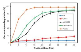
Insights into the degradation of carbamazepine using a continuous-flow non-thermal plasma: kinetics and comparison with UV-based systems
