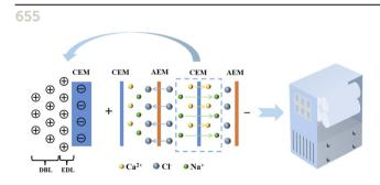
Selective removal of Ca<sup>2+</sup> from brackish water by electrodialysis desalination: process optimization and application
