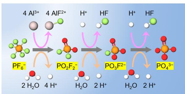
Kinetics and mechanism of hydrolysis of  $\text{PF}_6^-$  accelerated by  $\text{H}^+$  or  $\text{Al}^{3+}$  in aqueous solution
