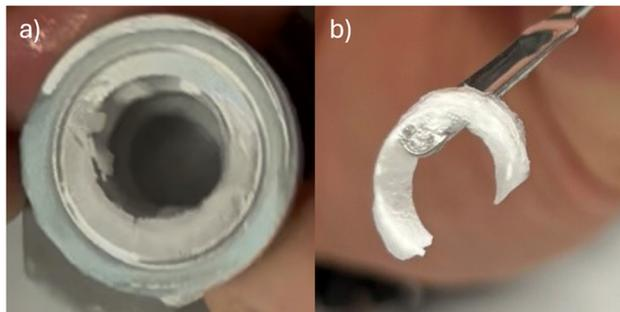
**Fig. 5** Clathrate-based desalination experiment with a 17.8 wt% solution KAc at 60 bar CH<sub>4</sub> and -15 °C. a) Inside of the reactor with clathrate creeping phenomenon visible at reactor wall. b) Clathrate hydrate separated from brine, facilitated by the creeping phenomenon.
