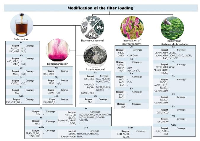
Fig. 3 Types of filter material coatings.
