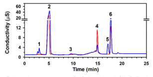
Fig. 3 Ion chromatograms at (red) 0 min and (blue) 7 min of irradiation ( $\lambda \geq$  295 nm) for control A at pH 7.0 for 30  $\mu M$  iohexol with 5.5 mg  $L^{-1}$  ClO<sup>-</sup>. Retention times ( $t_r$ ) for identified eluting species (see Table S2) are as follows: (1) iodate,  $t_r = 2.68$  min; (2) chloride,  $t_r = 4.60$ min; (3) chlorate,  $t_r = 9.93$  min; (4) sulfate,  $t_r = 14.85$  min; (5) iodide,  $t_r$ = 17.09 min; and (6) thiosulfate,  $t_r$  = 17.55 min.
