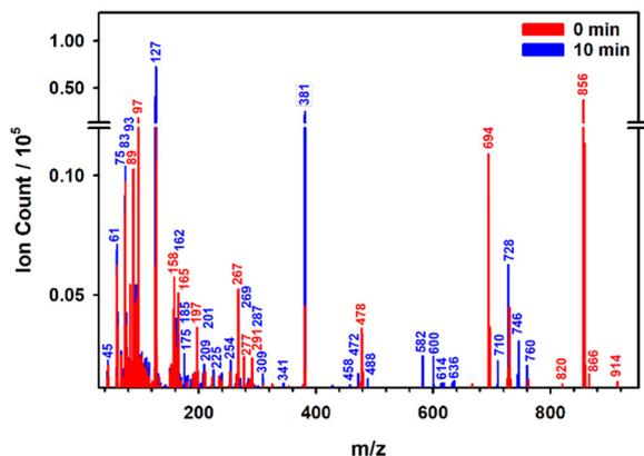
Fig. 4 Electro spray ionization-mass spectrometry (ESI-MS) analysis of experiment with 30  $\mu\text{M}$  iohexol, 3.0  $\text{mg L}^{-1}$  humic acids, and 5.5  $\text{mg L}^{-1}$   $\text{ClO}^-$  at pH 7.0 after (red) 0 and (blue) 10 min irradiation ( $\lambda_{\text{cut-off}} \geq 295$  nm). The  $m/z$  values are labeled in colors corresponding to the spectra with the largest intensity. Each spectrum was corrected by subtracting the corresponding solvent background.
