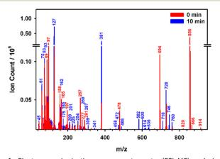
Fig. 4 Electrospray ionization-mass spectrometry (ESI-MS) analysis of experiment with 30  $\mu M$  iohexol, 3.0 mg  $L^{-1}$  humic acids, and 5.5 mg  $L^{-1}$ ClO<sup>-</sup> at pH 7.0 after (red) 0 and (blue) 10 min irradiation ( $\lambda_{cut-off} \ge 295$ nm). The m/z values are labeled in colors corresponding to the spectra with the largest intensity. Each spectrum was corrected by subtracting the corresponding solvent background.
