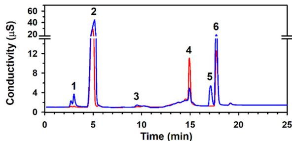
Fig. 3 Ion chromatograms at (red) 0 min and (blue) 7 min of irradiation ( $\lambda \geq 295$  nm) for control A at pH 7.0 for 30  $\mu\text{M}$  iohexol with 5.5  $\text{mg L}^{-1}$   $\text{ClO}^-$ . Retention times ( $t_r$ ) for identified eluting species (see Table S2) are as follows: (1) iodate,  $t_r = 2.68$  min; (2) chloride,  $t_r = 4.60$  min; (3) chlorate,  $t_r = 9.93$  min; (4) sulfate,  $t_r = 14.85$  min; (5) iodide,  $t_r = 17.09$  min; and (6) thiosulfate,  $t_r = 17.55$  min.
