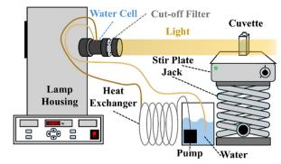
Scheme 1 Photochemical setup with a 1.0 kW Xe (Hg) lamp filtered through water to remove infrared radiation, and equipped with a cutoff filter at  $\lambda_{\text{cut-off}} \ge 295$  nm.
