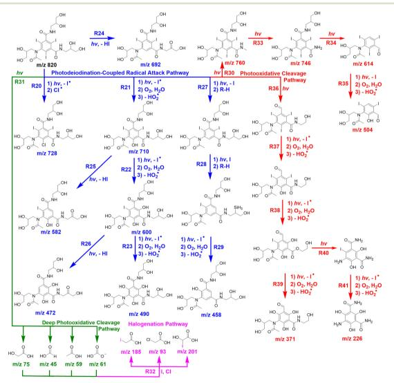
Scheme 3 Proposed irradiation/chlorination mechanism of iohexol transformation with color-coded observed *m/z* values corresponding to (blue) photodeiodination-coupled radical attack, (red) photooxidative cleavage, (green) deep photooxidative cleavage, and (pink) halogenation pathways.
