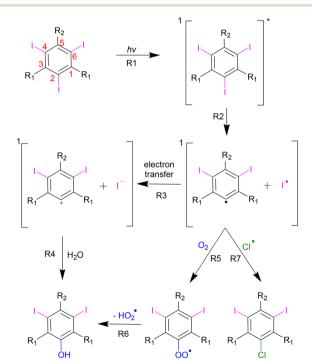
Scheme 2 Proposed deiodination of iohexol via direct photolysis.
