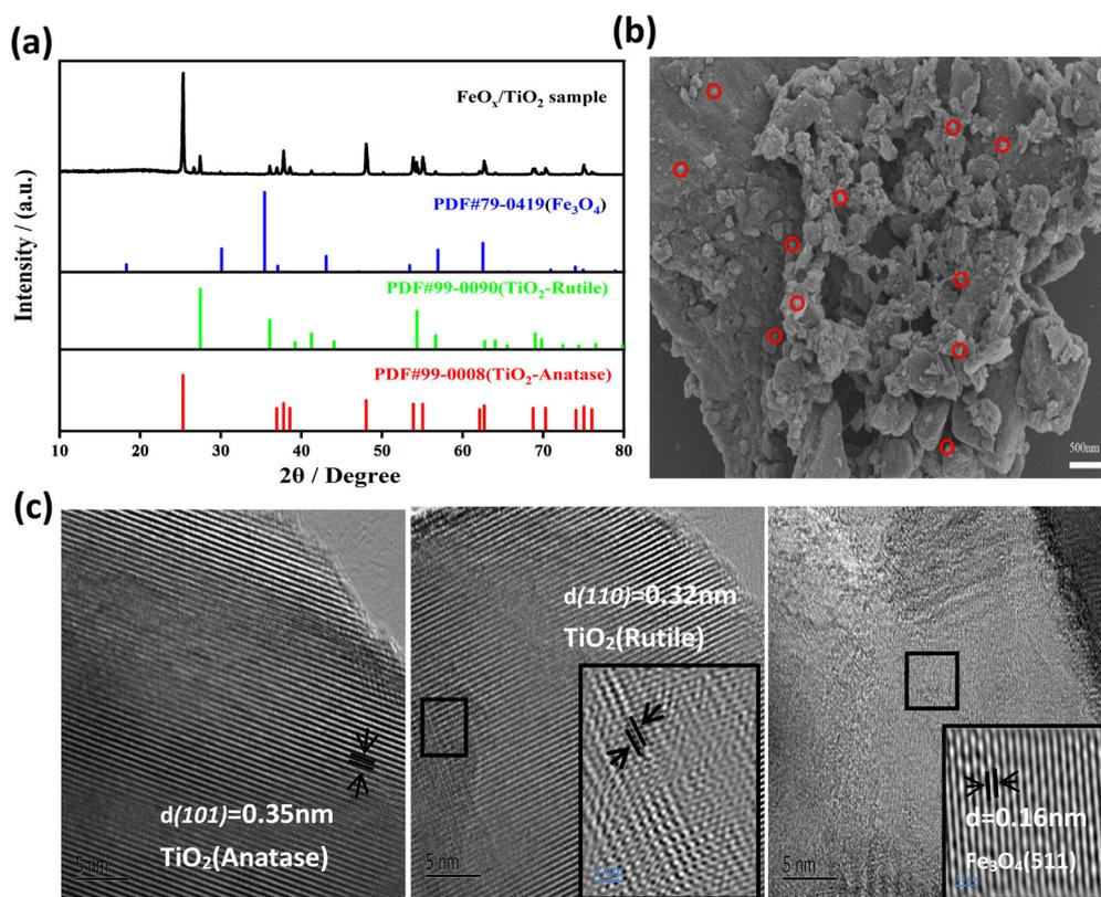
Fig. 3 (a) PXRD curves, (b) SEM image (red circles:  $\text{FeO}_x$  particles on the support), and (c) TEM images of the  $\text{FeO}_x/\text{TiO}_2$  catalyst sample (the inset figures are enlarged versions of the rectangular zoomed areas).
