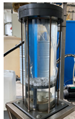
Fig. 2 Scheme of the experimental system (left) and photograph of the column (right): T, feed tank; V1, cutoff ball valve; V2, control diaphragm valve; S1 and S2, sample valves; P, circulating pump (with speed controller SC); FI, flow meter; DPI, differential pressure sensor; C, column.
