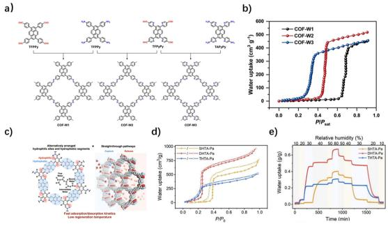
Fig. 6 (a) Schematic representation for the synthesis of COF-W1, COF-W2, and COF-W3. (b) Water adsorption isotherms of COF-W1, COF-W2, and COF-W3.<sup>26</sup> (c) Schematic illustration of DHTA-Pa COF for fast water capture/release and low-temperature regeneration. (d) Water sorption isotherms of SHTA-Pa COF, DHTA-Pa COF, and THTA-Pa COF at 298 K. (e) Dynamic water vapor adsorption-desorption kinetics of SHTA-Pa COF, DHTA-Pa COF, and THTA-Pa COF.35
