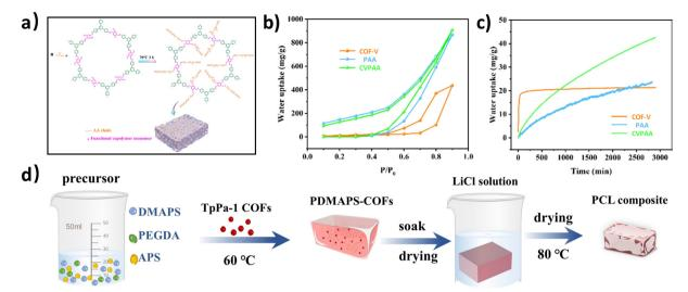
Fig. 8 (a) The reaction mechanism for the synthesis of CVPAA. (b) Water vapor adsorption isotherms of COF-V, PAA and CVPAA. (c) Water uptake performance of COF-V, PAA and CVPAA at 25 °C and 38% RH.<sup>67</sup> (d) Schematic representation of the fabrication process of the PCL hydrogel.<sup>47</sup>
