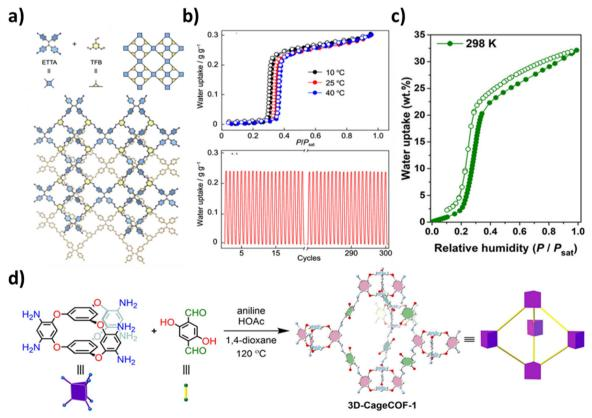
Fig. 3 (a) The synthesis scheme and simulated structure of COF-432. (b) Water isotherms and water cycling stability tests of COF-432 at different temperatures.<sup>25</sup> (c) Water vapor sorption isotherms for 3D-CageCOF-1. (d) Scheme for the synthesis of 3D-CageCOF-1 from Cage-6-NH2 and DHTPA (C: white, N: blue, O: red).<sup>24</sup>
