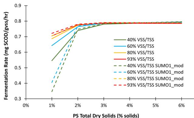
**Fig. 3** Generic benchmark plant model results with calibrated kinetic parameters for fermentation of 100% PS at varying VSS/TSS% and solids concentrations in a typical range for PS. Solid lines show results of SUMO1 model and dashed lines show results of SUMO1\_mod SUMO1 model.
