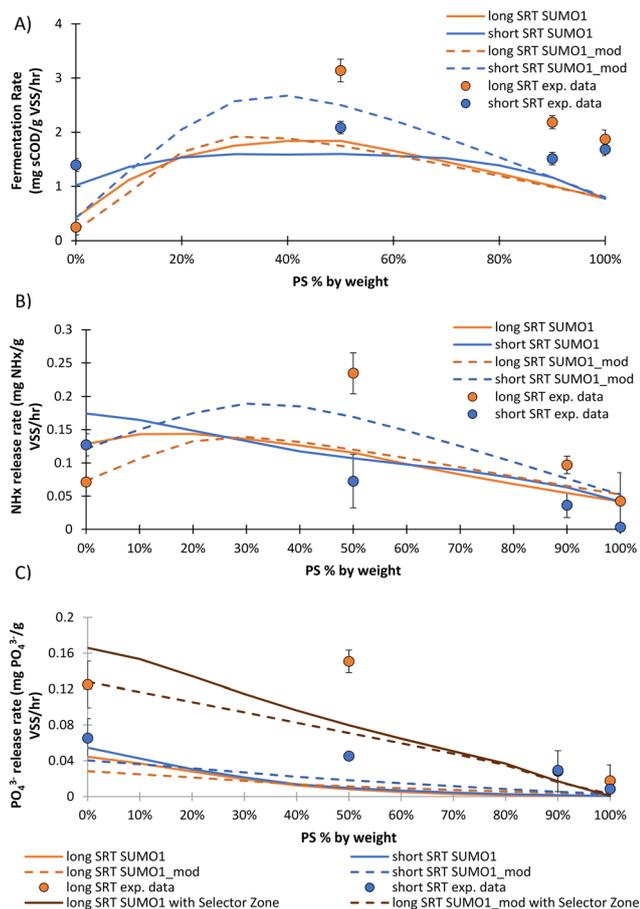
**Fig. 5** A) Fermentation rate as a function of % PS content by weight. B) NHx rerelease per g VSS as a function of % PS in the blend by weight. C)  $PO_4^{3-}$  rerelease per g VSS as a function of % PS in the blend by weight  $PO_4^{3-}$  release shown with a generic benchmark plant model with and without a selector zone (and therefore PAOs). Experimental data shown as data points, solid lines show the SUMO1 model and dashed lines show the SUMO1\_mod model. Both long SRT and short SRT shown.
