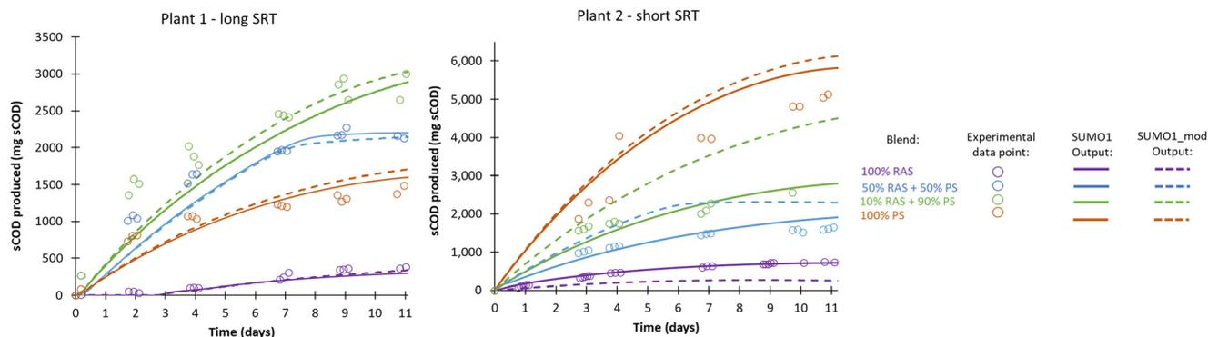
Fig. 2 sCOD yield data for plant 1 and 2 across different blends of batch experiments. Dots shown for experimental calibration data. Solid lines show calibrated SUMO1 model sCOD yield, and dashed lines show calibrated SUMO1\_mod model sCOD yield.
