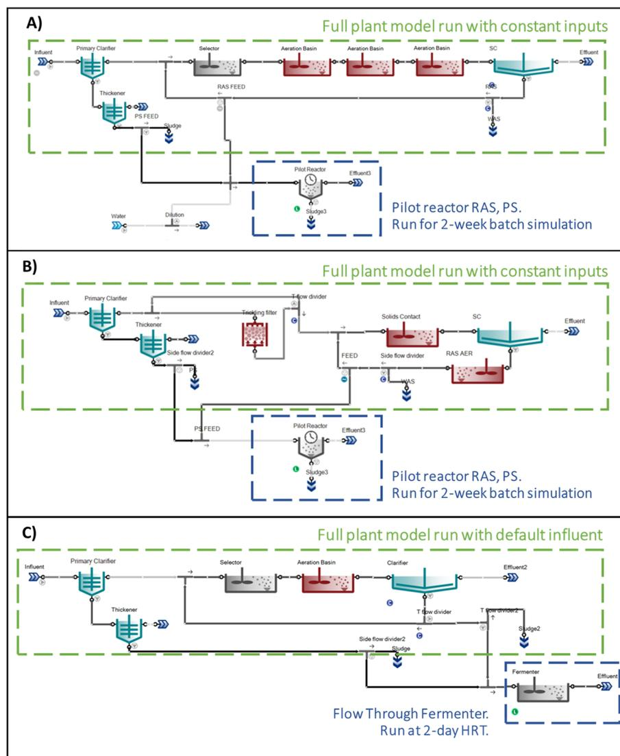
**Fig. 1** A) Model configuration for plant 1 nitrification–denitrification facility, long SRT 8–10 days with SBR fermenter, B) model configuration for plant 2 trickling filter facility with solids contact basin, short SRT 1–2 days with SBR fermenter and C) model configuration for generic benchmark plant used to test calibrated kinetic parameters analysis with flow through fermenter.
