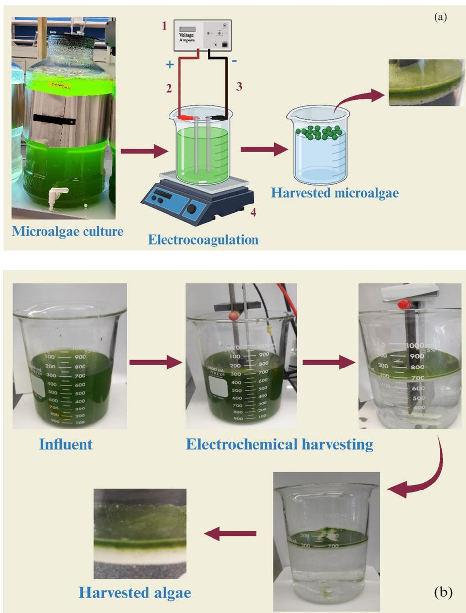
**Fig. 1** (a) The schematical diagram of electrocoagulation of algae (1: power supply, 2: anode, 3: cathode, 4: magnetic stirrer); (b) a real application of electrochemical algae harvesting.
