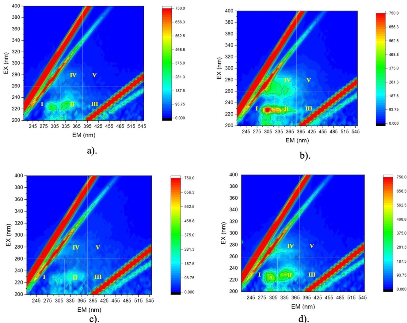
Fig. 9 Fluorescence excitation and emission matrix of the membrane cleaning solutions: (a) DW, (b) NaOH, (c) HCl and (d) citric acid for AEM.
