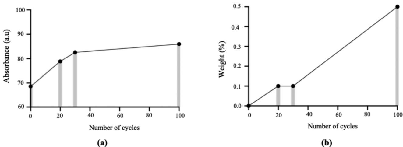
Fig. 5 FTIR absorbance values at 1670  $\text{cm}^{-1}$  over time, indicating the progression of organic fouling (a) and EDS elemental composition analysis showing calcium weight % on the membrane over time (b).
