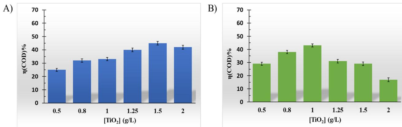
Fig. 5 Effect of TiO<sub>2</sub> concentration on the COD removal for (A) FUVL and (B) SUVL configurations.
