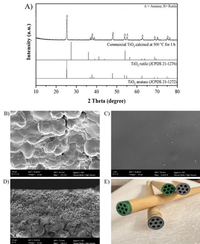
**Fig. 10** (A) XRD pattern of commercial  $\text{TiO}_2$ . SEM images of the multichannel  $\text{TiO}_2$  membrane used for the SPMR: (B) external top-view, (C) internal top-view, (D) cross-section and (E) picture of the multichannel  $\text{TiO}_2$  membrane.
