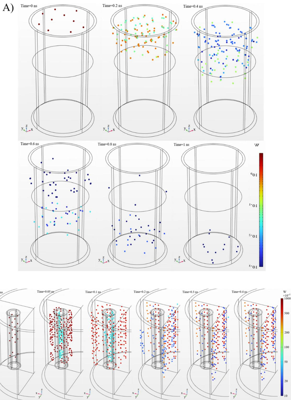
**Fig. 7** FEM results: (A) ray position and power on different simulation times (0–1 ns) for configuration A. (B) Ray position and power on different simulation times (0–1 ns) for configuration B (incident rays are “frozen” onto the two symmetry planes cutting the domain).
