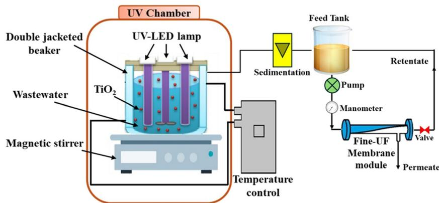
Fig. 3 Scheme of the slurry photocatalytic membrane reactor.
