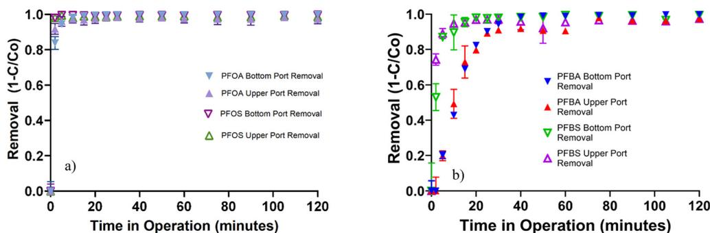
Fig. 5 Removal of an equal concentration PFAS mixture (PFOS |  $\text{Co} = 47\,000 \text{ ng L}^{-1}$ , PFOA |  $\text{Co} = 39\,000 \text{ ng L}^{-1}$ , PFBS |  $\text{Co} = 41\,000 \text{ ng L}^{-1}$ , PFBA |  $\text{Co} = 37\,000 \text{ ng L}^{-1}$ ) from synthetic groundwater using foam fractionation with a CTAB feed rate of  $1 \text{ mg min}^{-1}$ . Fig. 5a) shows removal for PFOA and PFOS and Fig. 5b) shows removal for PFBA and PFBS.
