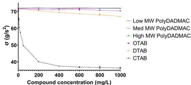
Fig. 3 Surface tension data for six potential cationic co-foaming agents in synthetic groundwater. Error bars represent standard deviation in surface tension data ( $n = 5$  replicates). Missing error bars are due to symbols size being greater than the error.
