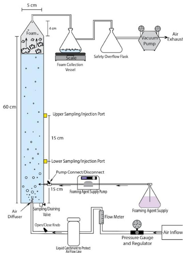
Fig. 1 Schematic diagram of the foam fractionation apparatus.
