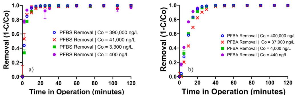
Fig. 6 Removal of a) PFBS and b) PFBA from synthetic groundwater in a foam fractionation system over four orders of magnitude concentration of PFAS in four compound mixture with a CTAB feed rate of  $1 \text{ mg min}^{-1}$ . Concentrations are averaged from measurements at both sampling ports as there was minimal concentration variations between ports.
