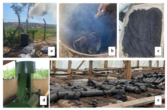
Fig. 1 (a) A metallic drum carbonisation kiln in use; (b) the carbonisation initiation with wood as a start-up fuel; (c) the produced faecal sludge char (ground); (d) the briquette extruder machine; and (e) the produced briquettes on drying racks (Lubigi Wastewater Treatment Plant, Kampala, Uqanda).
