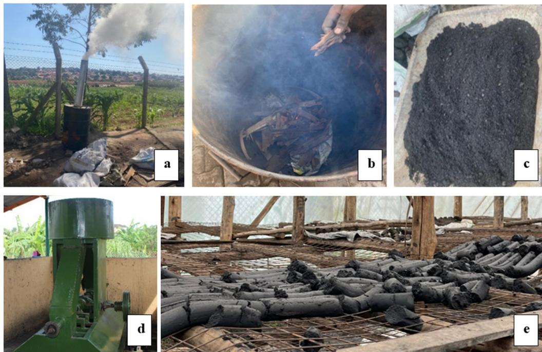
**Fig. 1** (a) A metallic drum carbonisation kiln in use; (b) the carbonisation initiation with wood as a start-up fuel; (c) the produced faecal sludge char (ground); (d) the briquette extruder machine; and (e) the produced briquettes on drying racks (Lubigi Wastewater Treatment Plant, Kampala, Uganda).
