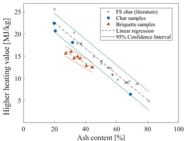
**Fig. 5** Correlation between higher heating value (MJ kg<sup>-1</sup>) and ash content (%) of char and briquette samples, with the inclusion of literature values for FS char samples.<sup>12,18,20,25</sup>
