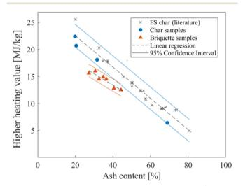
Fig. 5 Correlation between higher heating value (MJ  $\rm kg^{-1}$ ) and ash content (%) of char and briquette samples, with the inclusion of literature values for FS char samples. <sup>12,18,20,25</sup>
