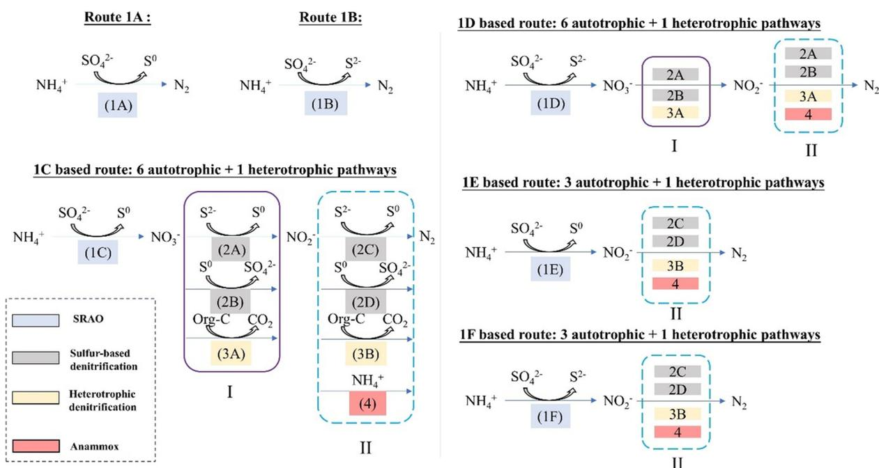
**Fig. 1** Extended hypothesis: overview of elementary SRAO reactions (1A, 1B, 1C, 1D, 1E, 1F) and of complex SRAO reactions with nitrogen gas as end product (18 combinations for autotrophic conditions and 4 combinations for heterotrophic conditions). Box I and box II group bioprocesses which are repeated. The reaction numbers and corresponding colours are consistent with Table 2; a full description is given in section 3.2.
