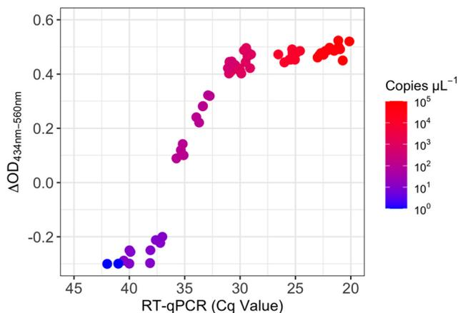
**Fig. 2** RT-LAMP detections ( $\Delta\text{OD}_{434-560\text{nm}}$ ) versus paired RT-qPCR cycle quantification (Cq) values of synthetic SARS-CoV-2 RNA. Each point represents an individual sample, with  $\Delta\text{OD}_{434-560\text{nm}}$  on the y-axis and Cq on the x-axis. The colour gradient indicates RNA concentrations of the synthetic reference material.
