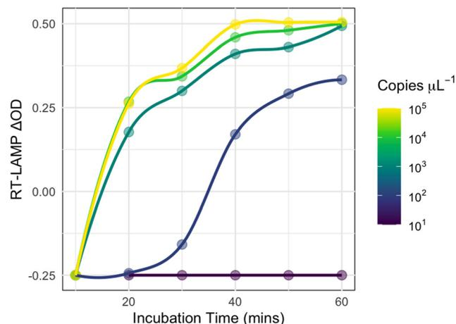
Fig. 1 Spectrophotometric  $\Delta\text{OD}_{434-560\text{nm}}$  measurements 10, 20, 30, 40, 50, and 60 minutes at 45 °C across five SARS-CoV-2 RNA concentrations ( $10^1$  to  $10^5$  copies per  $\mu\text{L}$ ). Points represent the average  $\Delta\text{OD}_{434-560\text{nm}}$  measured at each point ( $n = 10$ ), and the lines are smoothed trends generated using LOESS smoothing function in RStudio.
