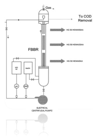
Fig. 1 Denitrification fluidized-bed bioreactor.
