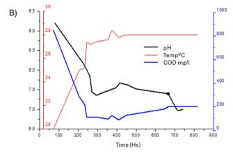
Fig. 6 Denitrification process in FBBRs: A) denitrification performance and B) monitored parameters: pH, T (°C), and COD.
