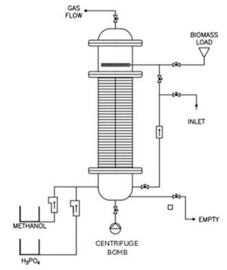
Fig. 2 Packed-bed bioreactor.
