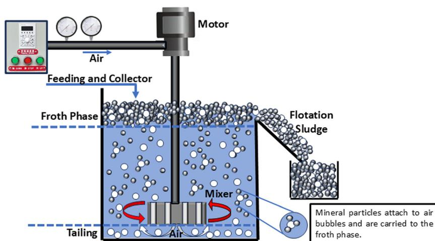
Fig. 2 Flotation experiment.
