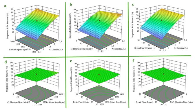
Fig. 7 Effect of factor interactions on SS removal response: (a) A-B interaction, (b) A-C interaction, (c) A-D interaction, (d) B-C interaction, (e) B-D interaction, and (f) C-D interaction.
