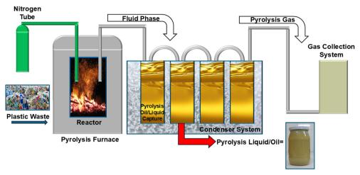
Fig. 1 Pyrolysis liquid/oil production in a pyrolysis system.
