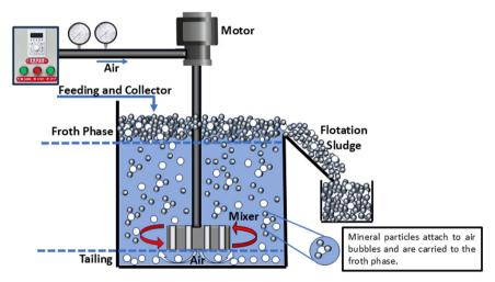
Fig. 2 Flotation experiment.
