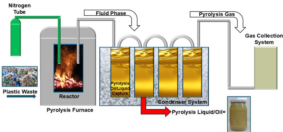
Fig. 1 Pyrolysis liquid/oil production in a pyrolysis system.
