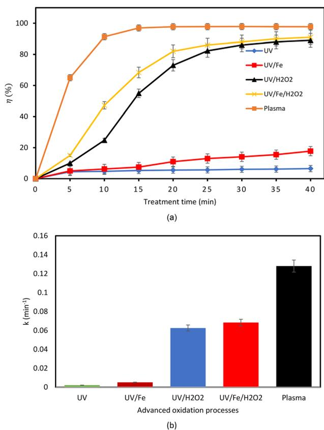
**Fig. 14** (a) Comparison of the different AOPs in terms of degradation efficiency. (b) Comparison of the different AOPs in terms of reaction kinetics (experimental conditions: volume of solution = 500 mL; initial CBZ concentration = 10 mg L<sup>-1</sup>).
