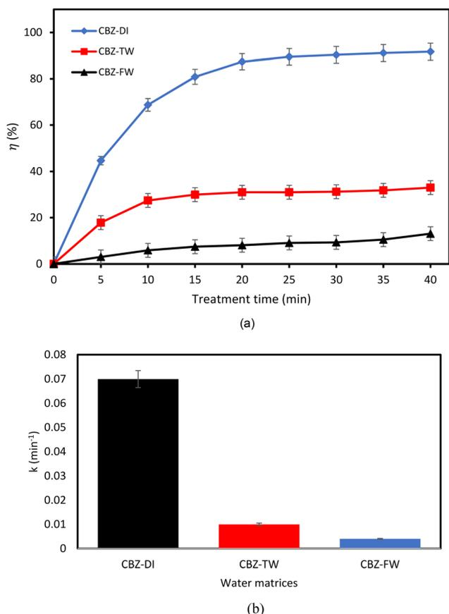
Fig. 13 (a) Effect of water matrices on degradation efficiency of CBZ. (b) Effect of water matrices on reaction rate for CBZ degradation (experimental conditions: CBZ initial concentration  $10 \text{ mg L}^{-1}$ ; voltage  $6 \text{ kV}$ ; frequency  $20 \text{ kHz}$ ).
