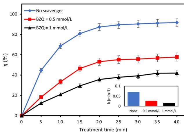
Fig. 10 Influence of *p*-benzoquinone on the degradation efficiency of CBZ (experimental conditions: CBZ initial concentration  $10 \text{ mg L}^{-1}$ ; voltage  $6 \text{ kV}$ ; frequency  $20 \text{ kHz}$ ).
