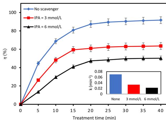
Fig. 9 Influence of isopropanol on the degradation efficiency of CBZ (experimental conditions: CBZ initial concentration 10 mg L<sup>-1</sup>, voltage 6 kV; frequency 20 kHz).
