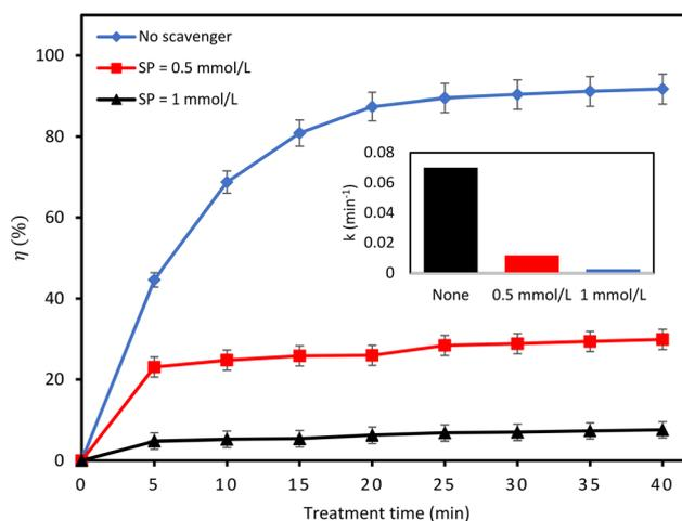
Fig. 12 Influence of sodium pyruvate on the degradation efficiency of CBZ (experimental conditions: CBZ initial concentration  $10 \text{ mg L}^{-1}$ ; voltage  $6 \text{ kV}$ ; frequency  $20 \text{ kHz}$ ).
