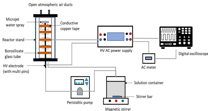
**Fig. 1** Experimental setup for the dielectric barrier discharge plasma system.
