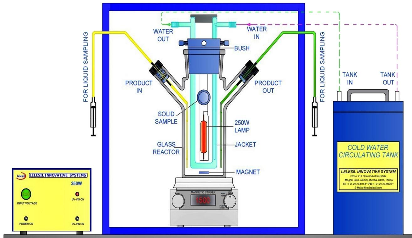
Fig. 2 Setup for the UV-based experiments.
