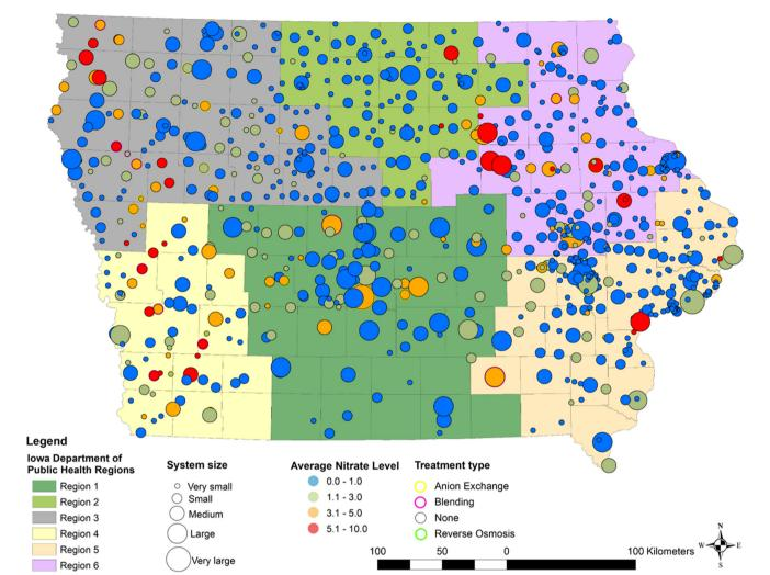
Fig. 5 Nitrate concentration averaged for 2012-2022 for each PWS in Iowa. Outline color indicates the type of nitrate removal process. Size of circle indicates system size. Underlying background color indicates Iowa Department of Public Health Regional Medical Coordination Centres.
