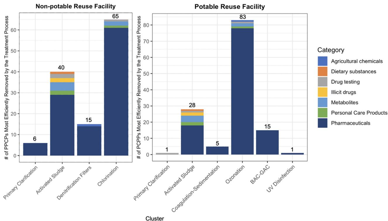
Fig. 3 The number of PPCPs in each cluster based on the C1 clustering method, *i.e.*, according to the most efficient individual treatment process contributing to removal of each PPCP across the treatment train.
