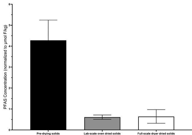
**Fig. 3** Average total PFAS concentration (normalized to  $\mu\text{mol F kg}^{-1}$ ) across pre-drying solids, lab-scale oven post-drying solids, and full-scale dryer post-drying solids. Samples taken in triplicate ( $n = 3$ ) and error bars represent standard deviation. Reprinted with permission. © The Water Research Foundation.<sup>39</sup>
