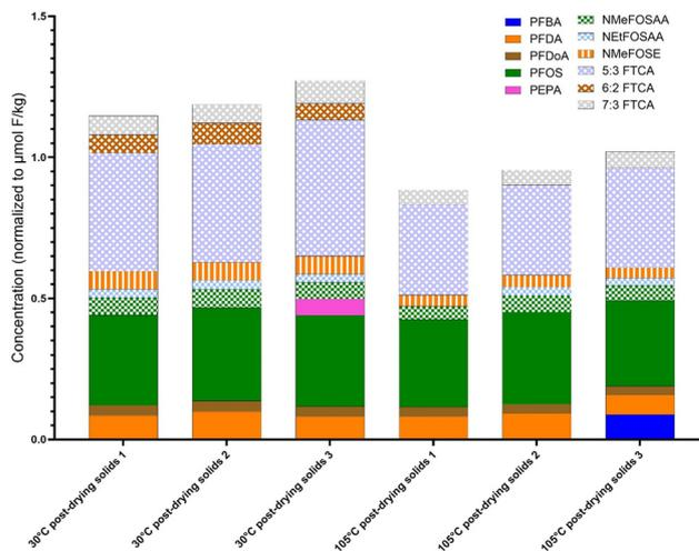
**Fig. 5** Drying at 105 °C decreased total PFAS concentration by 16% compared to drying at 30 °C. Water content of pre-drying solids was 99.8%. 30 °C and 105 °C drying of samples were conducted in triplicate ( $n = 3$ ). Reprinted with permission. © The Water Research Foundation.<sup>39</sup>
