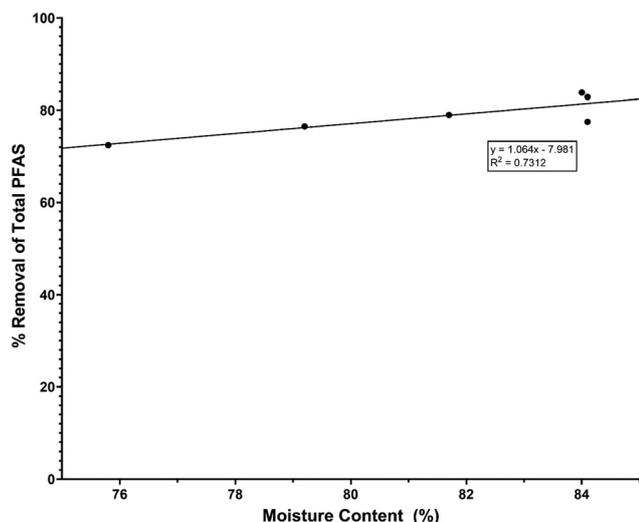
Fig. 6 Moisture content correlated to PFAS removal across sample sets. Reprinted with permission. © The Water Research Foundation.<sup>39</sup>
