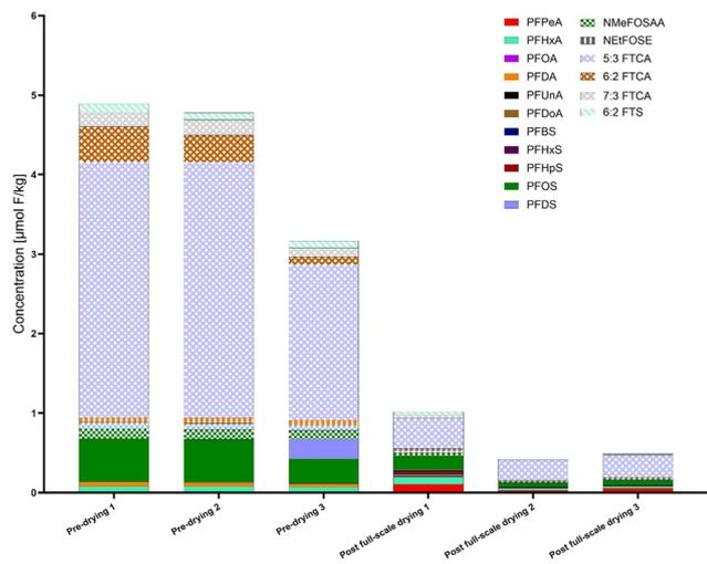
Fig. 1 Full-scale drying reduces measurable PFAS concentrations in biosolids. Samples were collected in triplicate ( $n = 3$ ). Reprinted with permission. © The Water Research Foundation.<sup>39</sup>
