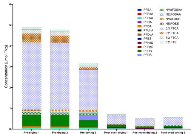
Fig. 2 Lab-scale oven drying at 105 °C reduces measurable PFAS concentrations in biosolids. Triplicate lab-scale oven drying experiments were conducted ( $n = 3$ ). Reprinted with permission. © The Water Research Foundation.<sup>39</sup>
