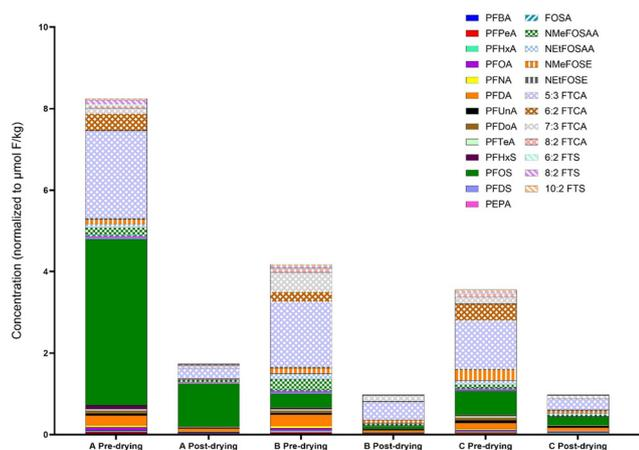
**Fig. 4** Lab-scale oven drying reduced measurable PFAS in samples from three different WRRFs. Reprinted with permission. © The Water Research Foundation.<sup>39</sup>
