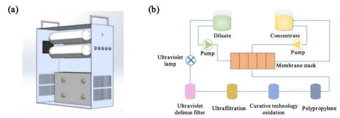
Fig. 3 (a) Guided ED integrated device and (b) water purification process flowchart.
