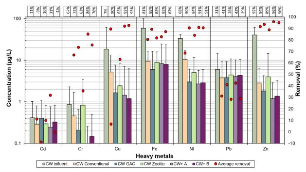
Fig. 3 Average concentrations in influent and CW effluents and removal of heavy metals in the CW influent and the effluent of the respective CWs with standard deviations (n = 24). The values indicated above the graph represent the average removal rate of the respective CWs in the order as depicted in the figure from left to right.
