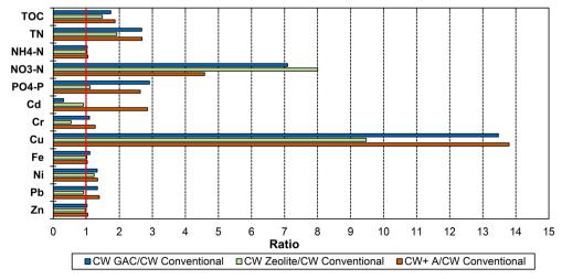
Fig. 5 Treatment efficiency expressed in ratio removal of  $CW_{Conventional}$  to  $CW_{GAC}$ ,  $CW_{Zeolite}$  and  $CW^+$  A. Values < 1 indicate better removal in  $CW_{Conventional}$  values > 1 better removal in the modified wetlands.
