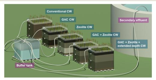
Fig. 1 Constructed wetland pilot setup at the STP Emschermündung in Dinslaken, Germany from left to right:  $CW_{Conventional}$   $CW_{GAC}$ ,  $CW_{Zeolite}$ ,  $CW^+$ A and  $CW^+$ B.
