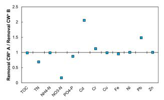
Fig. 8 Treatment efficiency of CW $^+$  A and CW $^+$  B expressed in ratio removal CW $^+$  A to removal CW $^+$  B. Values < 1 indicate better removal in CW $^+$  B, values > 1 better removal in CW $^+$  A.
