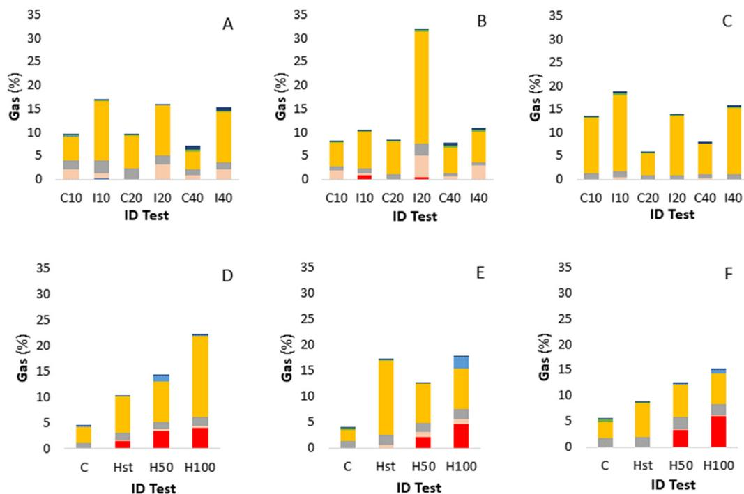
**Fig. 4** Gas composition (%) at the end of the hydrogenotrophic denitrification tests varying inoculum percentage (v/v) and hydrogen supply in the 1st (A and D), 2nd (B and E) and 3rd cycle (C and F): hydrogen (■), nitric oxide (■), methane (■), water (■), nitrogen (■), nitrous oxide (■) and carbon dioxide (■). The complement to 100% is represented by the argon gas used to flush the bottles at the beginning of the experiments.
