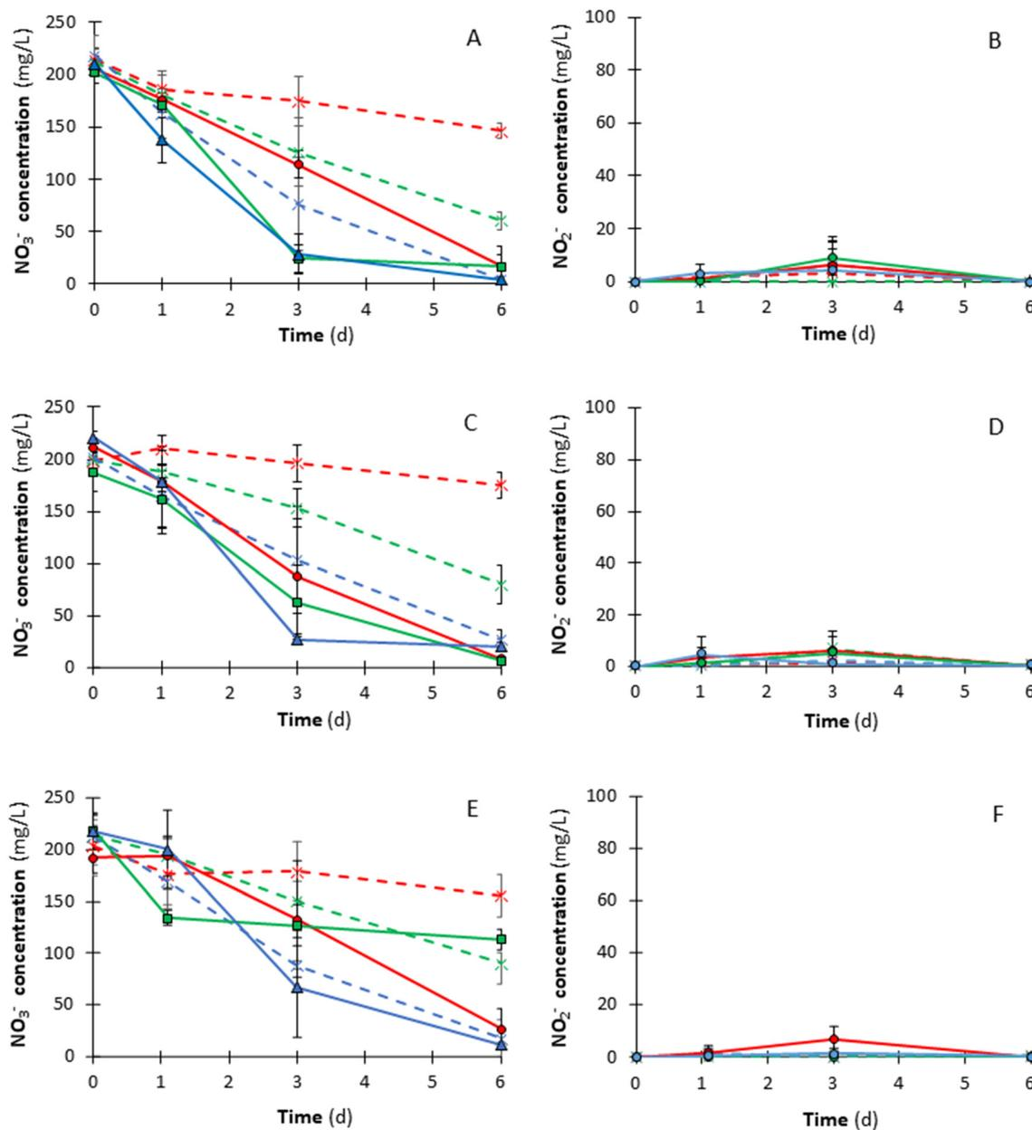
Fig. 2 Nitrate ( $\text{NO}_3^-$ ) (left column) and nitrite ( $\text{NO}_2^-$ ) (right column) concentration trend during the hydrogenotrophic denitrification tests across three cycles: the first cycle (A and B), second cycle (C and D), and third cycle (E and F). The tests were conducted using different inoculum percentages, *i.e.*, 10% (I10), 20% (I20) and 40% (I40) (v/v). Inoculum percentage tests: I10 (●), I20 (■), I40 (▲). Control tests: C10 (×), C20 (×), C40 (×).
