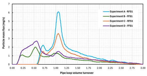
Fig. 4 Flushing stage 2 mass flux profiles measured at the outlet for exp. A - RFS1 (T1), exp. B - FFS1 (T3), exp. C - RFS1 (T1), and exp. D - FFS1 (T3).
