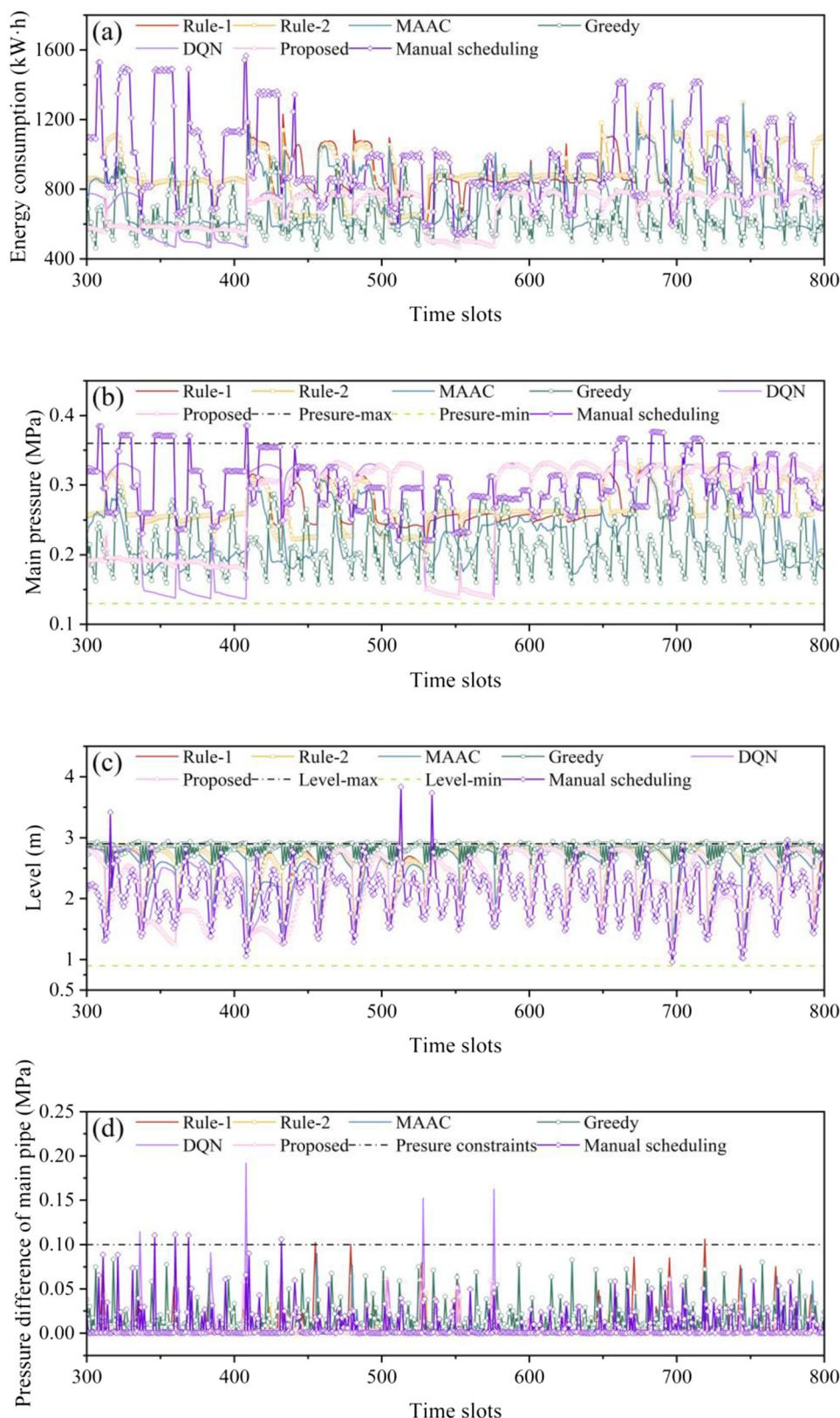
**Fig. 3** Performance details among all schemes for WIPS 1. (a) Energy consumption, (b) main pressure, (c) level, and (d) pressure difference of the main pipe.
