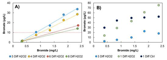
Fig. 9 A) Plant B bromide spike testing at 1.1 (O<sub>3</sub>-NO<sub>2</sub>): TOC, 1:1 H<sub>2</sub>O<sub>2</sub>: O<sub>3</sub> with 3, 4, 6, & 8 diffusers and B) repeated bromide spike testing with a single diffuser and a no peroxide control condition.
