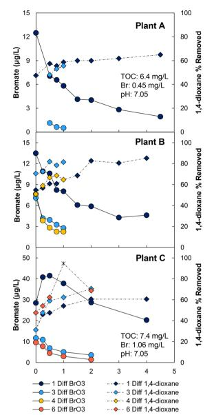
Fig. 4 Bromate formed and 1,4-dixoane removed at a fixed ozone dose of 0.8 (O<sub>3</sub>-NO<sub>2</sub>): TOC. Temp: 19-21 °C. Lines added for visual aid. The asterisk symbol represents removal calculated using ½ the MRL for a value below detection.
