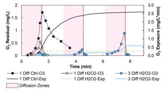
Fig. 5 Example ozone residual (-O<sub>3</sub>) and exposure (-Exp) profile for plant A effluent at 0.8  $O_3$ : TOC (7.0 mg  $L^{-1}$   $O_3$ , 2.32 mg  $L^{-1}$  to each with three diffusers). Ozone exposure was calculated as the area under the ozone residual profiles. For the single diffuser control condition (Ctrl) the 1st order ozone decay rate was calculated, then the decay curve was extended and integrated until ozone had completely
