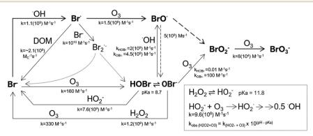
Fig. 1 Bromate formation pathways and mechanisms of mitigation by hydrogen peroxide. Closely adapted from Buffle *et al.*,<sup>25</sup> with reactions and rate constants from Lei *et al.*,<sup>26</sup> and von Sonntag and von Gunten.<sup>27</sup>
