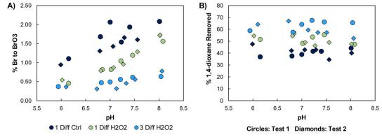
Fig. 7 A) Molar conversion of bromide to bromate and B) 1,4-dioxane removed in plant B secondary effluent at a fixed ozone dose of 0.8 (O<sub>3</sub>- $NO_2^{-1}$ : TOC, 20 °C. Test 1: 8.56 mg L<sup>-1</sup> TOC, 0.163 mg L<sup>-1</sup> Br, Test 2: 9.8 mg L<sup>-1</sup> TOC, 0.365 mg L<sup>-1</sup> Br.
