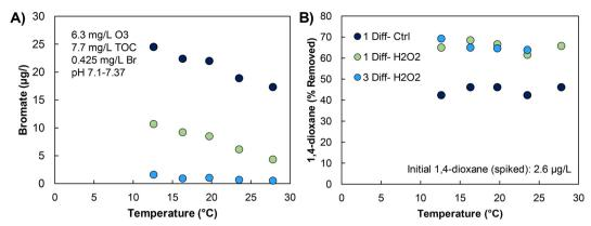
Fig. 10 A) Bromate formed and B) 1,4-dioxane removed in plant A effluent from 12–28 °C at 0.8  $(O_3-NO_2)$ : TOC. 4.25 mg L<sup>-1</sup> H<sub>2</sub>O<sub>2</sub> when used (1:1 H<sub>2</sub>O<sub>2</sub>: O<sub>3</sub>).
