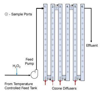
Fig. 2 Pilot ozone contactor diagram.
